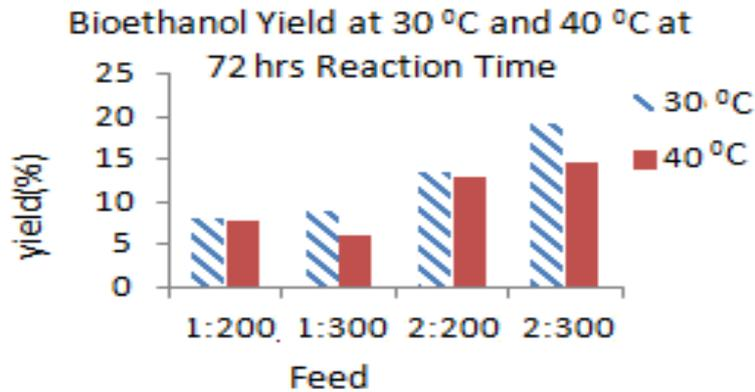
Fig. 3 Effect of feed ratio on bioethanol yield at various temperatures
