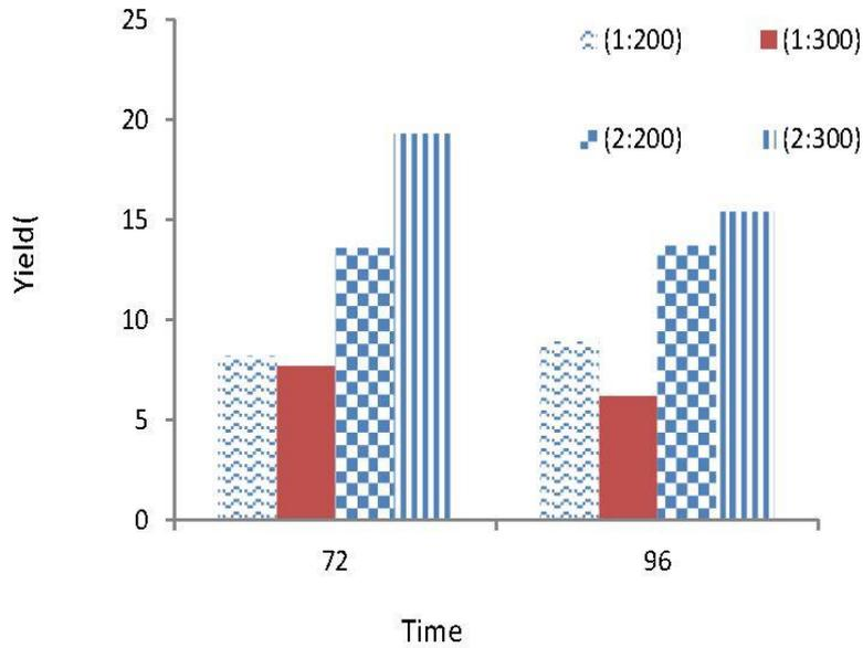
Fig. 2 Effect of reaction time on bioethanol yield at various feed loading
