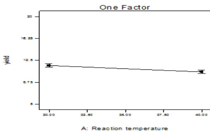
Fig. 5 Graph of yield against reaction temperature
