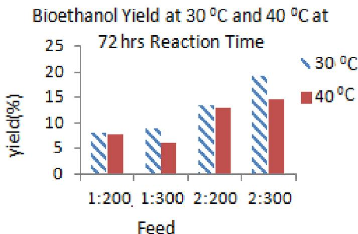
Fig. 1 Effect of temperature on bioethanol yield at various feed ratios
