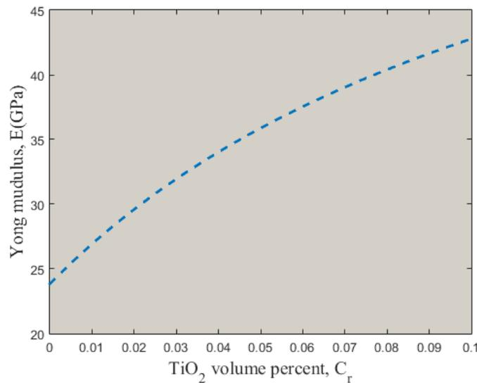
Fig. 1 The effect of  $TiO_2$  nanoparticles on the elastic modulus of the concrete
