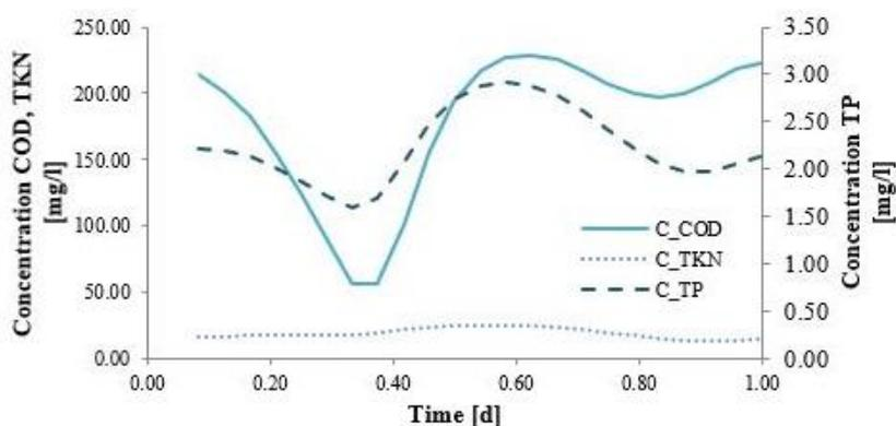
Fig. 5 Modeled influent concentration profiles of COD, TKN and TP for WWTP Butile/Sarajevo
