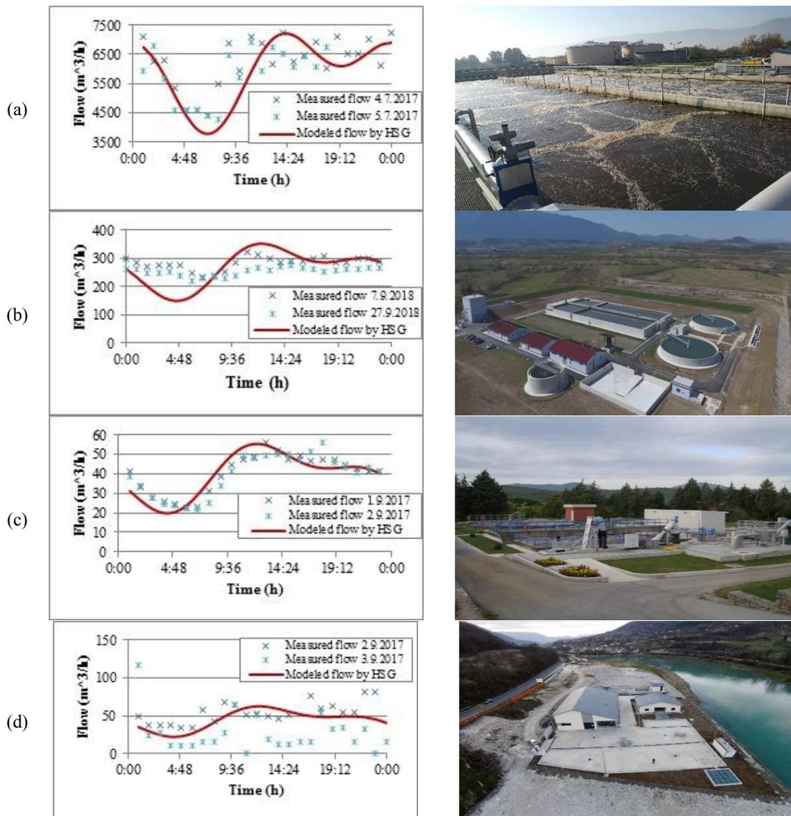
Fig. 4 Charts with comparison of measured and modeled inflow (left side) and view\* of WWTPs in B&H (right side): (a) Sarajevo - 600.000 PE, (b) Bihac - 55.000 PE, (c) Ljubuski - 6.000 PE, (d) Konjic - 5.000 PE
