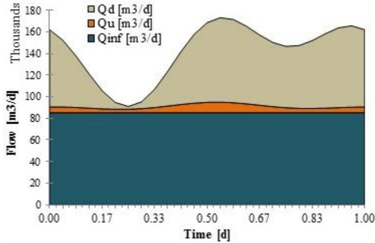
Fig. 2 Influent discharge, composed of three wastewater components (infiltration water ( $Q_{inf}$ ), urine flow ( $Q_u$ ) and domestic wastewater without urine ( $Q_d$ ))
