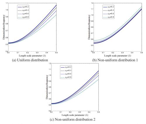
Fig. 4 Normalized frequency of double-coupled nanoplate against strain gradient parameter for different porosity distributions ( $K_0=50$ , a/h=10,  $\Delta T=0$ ,  $K_w=0$ ,  $K_p=0$ ,  $\mu=0.2$ )
