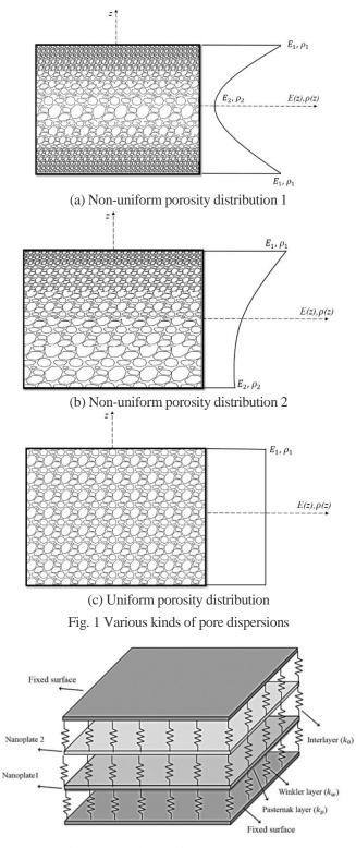
Fig. 2 A double-coupled nanoplate system
