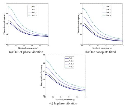
Fig. 3 Normalized frequency of double-coupled nanoplate against nonlocal and strain gradient parameters (a/h=10, K<sub>w</sub>=0, K<sub>p</sub>=0,  $\Delta$ T=0, K<sub>0</sub>=50,  $e_0$ =0.5)
