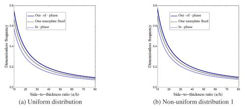
Fig. 6 Normalized frequency of double-coupled nanoplate against side-to-thickness ratio for different types of vibration ( $e_0=0.5$ ,  $K_w=25$ ,  $K_p=5$ ,  $\mu=0.2$ ,  $\Delta T=0.1$ ,  $K_0=100$ )
