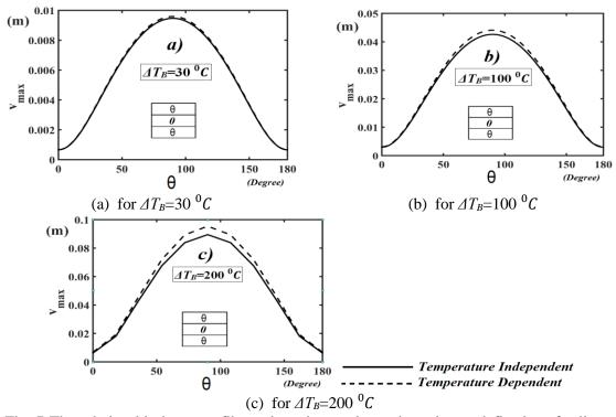
Fig. 7 The relationship between fiber orientation angles and maximum deflections for linear and nonlinear solution for the stacking sequence  $[\theta/0/\theta]$
