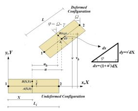
Fig. 2 The kinematics and coordinates of the beam element in the Lagrangian approach
