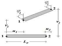
Fig. 3 Finite beam element model
