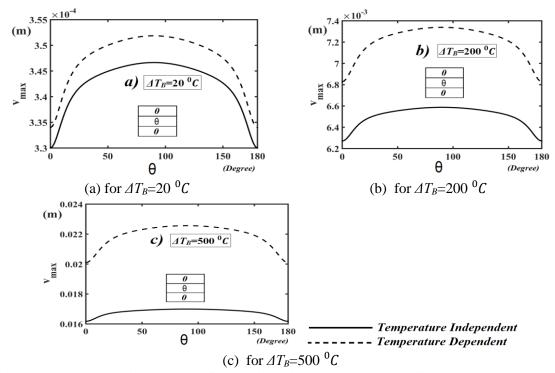
Fig. 6 The relationship between fiber orientation angles and nonlinear maximum thermal deflections with temperature dependent and independent physical properties for  $[0/\theta/0]$
