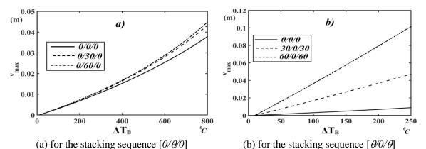
Fig. 4 The maximum transversal displacements  $v_{max}$  versus temperature rising  $\Delta T_B$  with different fiber orientation angles in the temperature dependent physical properties.
