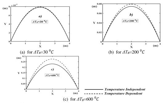
Fig. 8 The difference between temperature dependent and independent physically properties on the nonlinear deflected configuration for the stacking sequence 30/0/30
