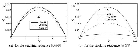
Fig. 5 Thermal nonlinear deflected configuration of the laminated beam for different values of the fiber orientation angles for  $\Delta T_B=500$  <sup>o</sup>C
