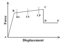
Fig. 6 Plastic hinge behavior according to FEMA 356 (Computers & Structures, Inc. 2016)
