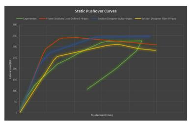
Fig. 12 Static pushover curves: Experimental vs. SAP2000 models
