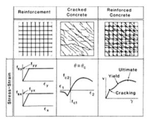
Fig. 4 The Modified compression filed theory for membrane elements (Vecchio and Collins 1986)
