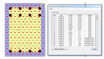
Fig. 11 Section C-C generated fibers
