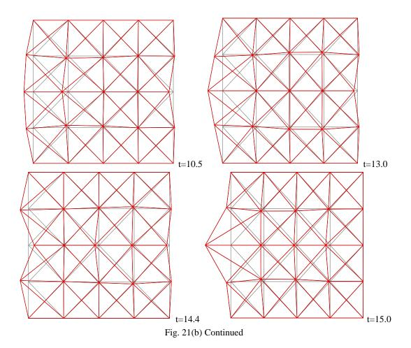
From Fig. 21 (but even more from their animation), it is visible that in the Kelvin model a strain wave propagates through the material from one side of the sample to the other, causing finally material eruption at the exit; in the Maxwell model, a strain wave is reflecting from sides eventually superposing and causing eruption at the exit.
