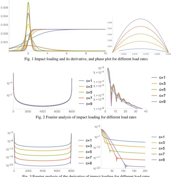
Fig. 3 Fourier analysis of the derivative of impact loading for different load rates
