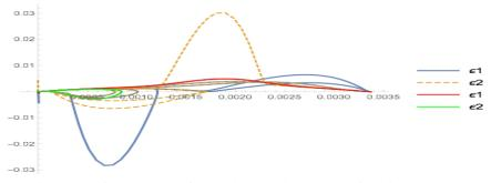
Fig. 10 Kelvin, phase plot for one large and one small viscosity parameter
