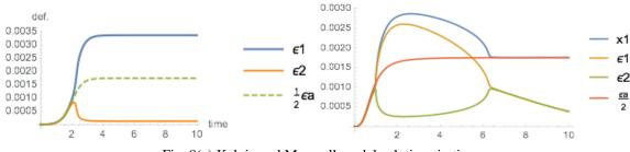
Fig. 8(a) Kelvin and Maxwell model solutions in time
