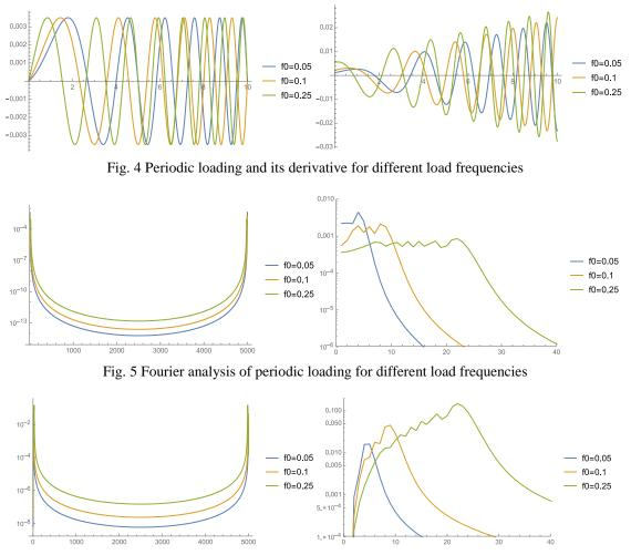
Fig. 6 Fourier analysis of the derivative of periodic loading for different load frequencies
