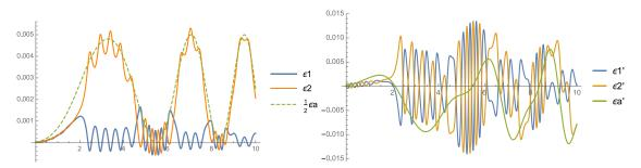
Fig. 17(a) Kelvin, deformations and its derivative in time
