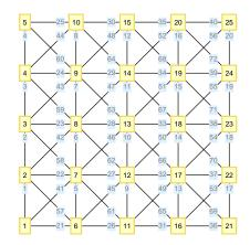
Fig. 19 Kelvin and Maxwell structure models for analysis
