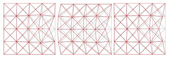
Fig. 20(b) Maxwell structure under fast impact, after t=0.8, t=1.8 and t=3.3 time units
