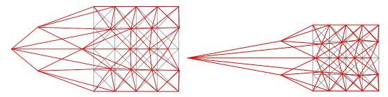
Fig. 20(a) Kelvin structure under slow and fast impact, after t=20 and t=4 time units
