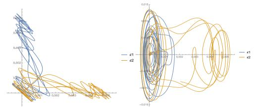
Fig. 17(b) Kelvin, deformations in parametric space ( $\varepsilon_{e1}$ vs.  $\varepsilon_{e2}$ )
