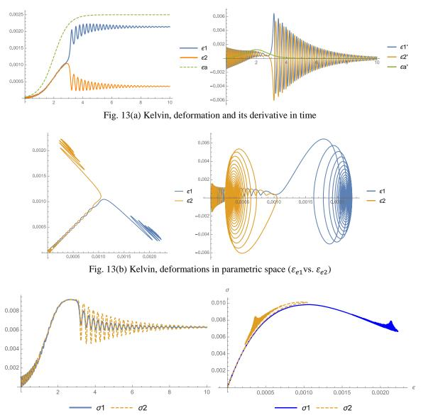
Fig. 13(c) Kelvin, stress in time and in parametric space ( $\sigma$  vs.  $\varepsilon$ )
