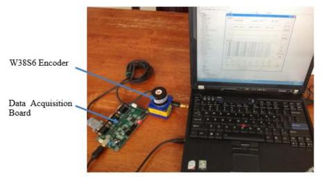
Fig. 3 W38S6 Wire draw Encoder system
