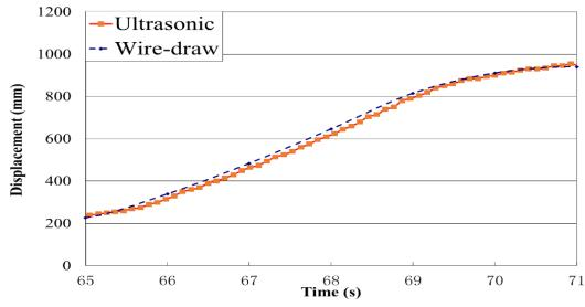
Fig. 12 Displacement measured by the ultrasonic and the wire draw sensing systems (65s to 71s)
