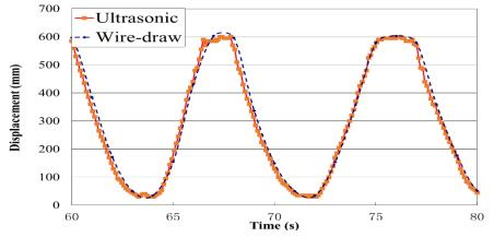
Fig. 7 Displacement measured by the ultrasonic and the wire draw sensing systems (60s to 80s)
