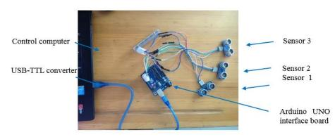
Fig. 2 Ultrasonic distance sensing system with three distance sensors
