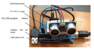
Fig. 1 An Ultrasonic sensing system with US-100 module
