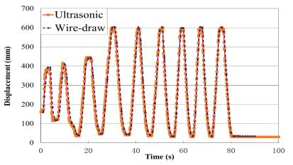
Fig. 6 Displacement measured by the ultrasonic and the wire draw sensing systems
