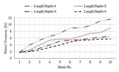
Fig. 7 Changes of natural frequencies for different L/D ratios
