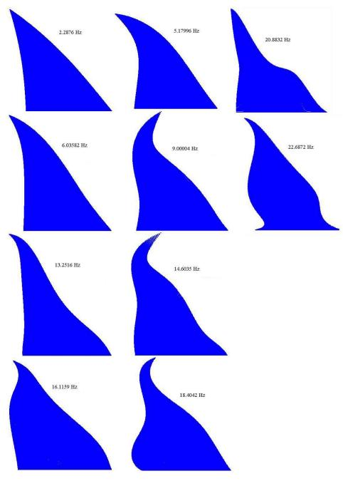
Fig. 12 Mode shapes of triangular Dam (one element)
