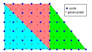
Fig. 15 Reservoir model with 21 node-33 gauss point element (L/D=1)
