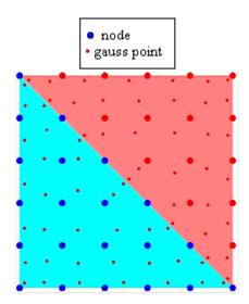
Fig. 14 Reservoir model with 21 node-33 gauss point element (L/D=1)
