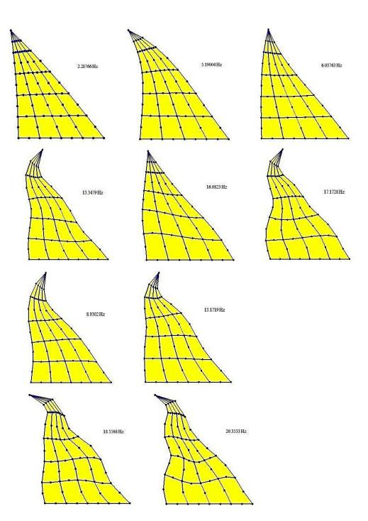
Fig. 9 Mode shapes of triangular Dam (20 elements)
