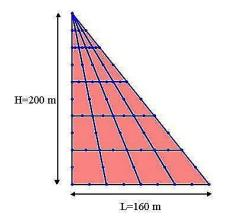
Fig. 8 Dam modelled by eight-node triangular elements
