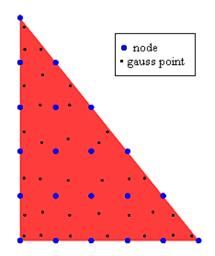
Fig. 13 Dam model with 21 node-33 gauss point element
