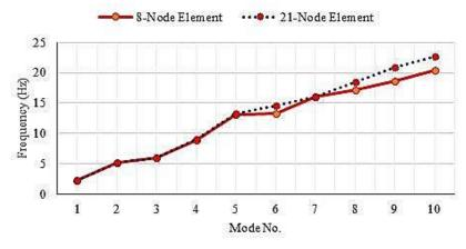
Fig. 11 Comparison between frequencies of dam models
