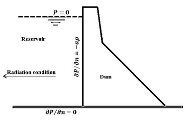
Fig. 1 Solid-fluid common boundary
