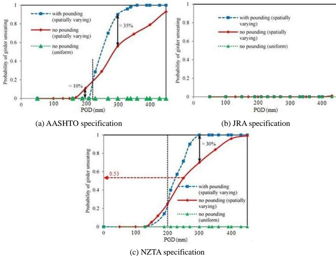
Fig. 3 Comparison of fragility curves of bridge girder unseating with and without pounding when subjected to uniform and spatially varying ground motions, excluding effects of ground motion characteristics and coherency loss, i.e. data for all cases considered are used
