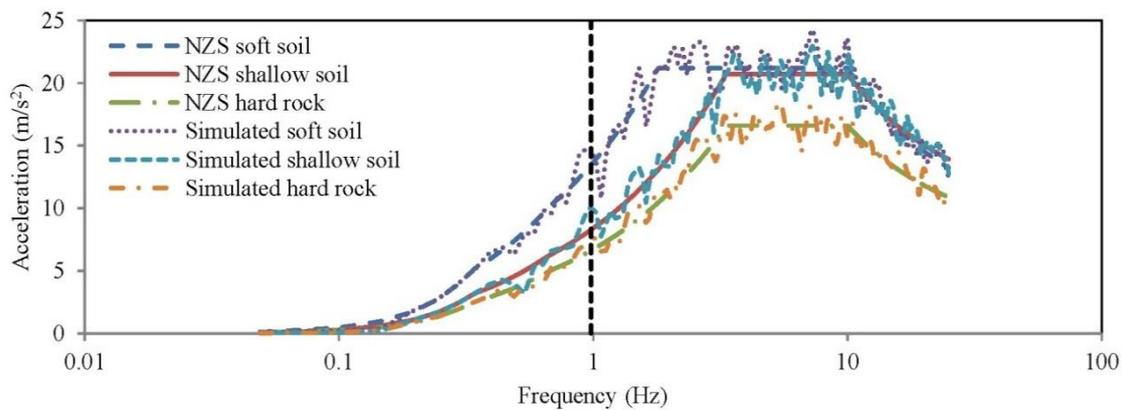
Fig. 2 Design and response spectra of simulated ground motions
