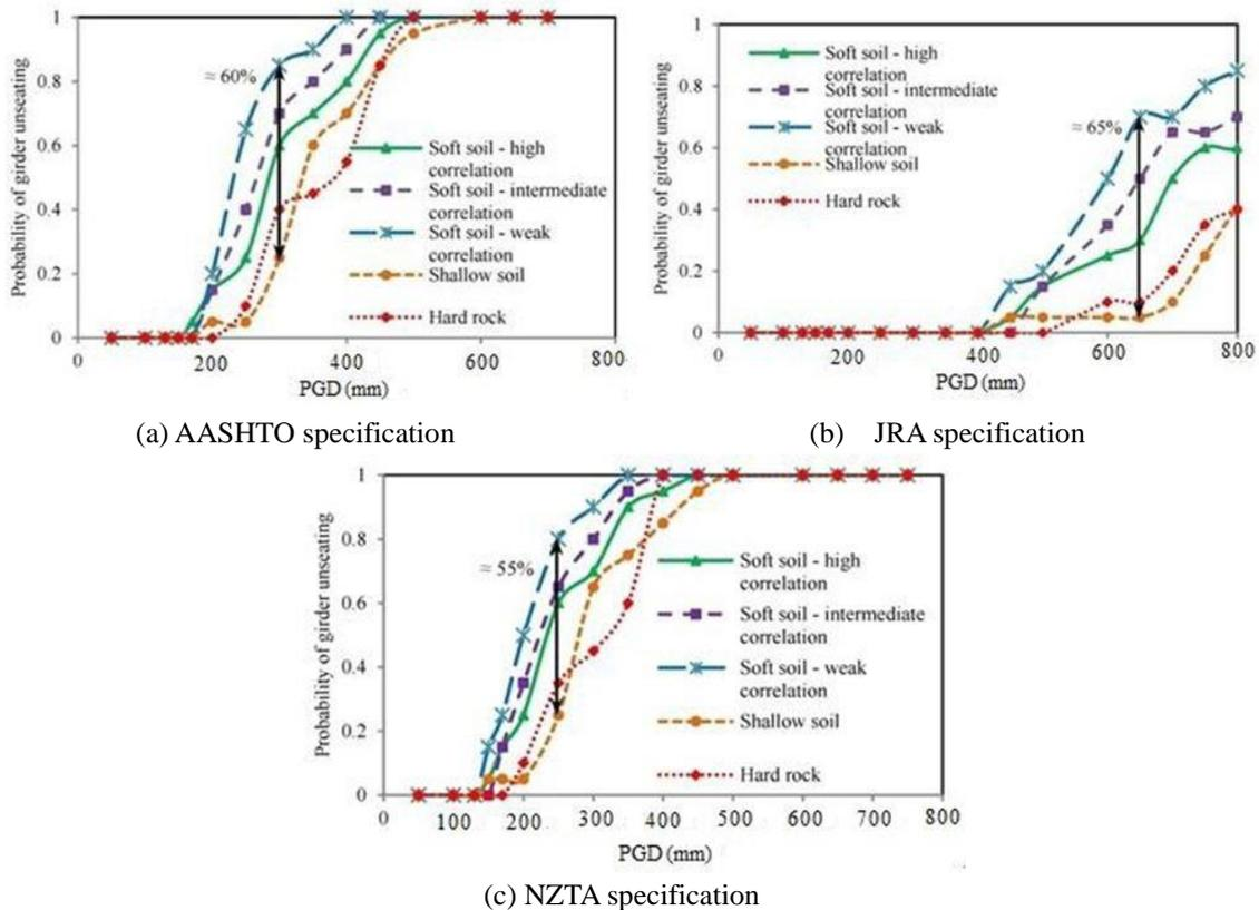
Fig. 5 Fragility curves of bridge for ground excitations based on various soil conditions without considering pounding
