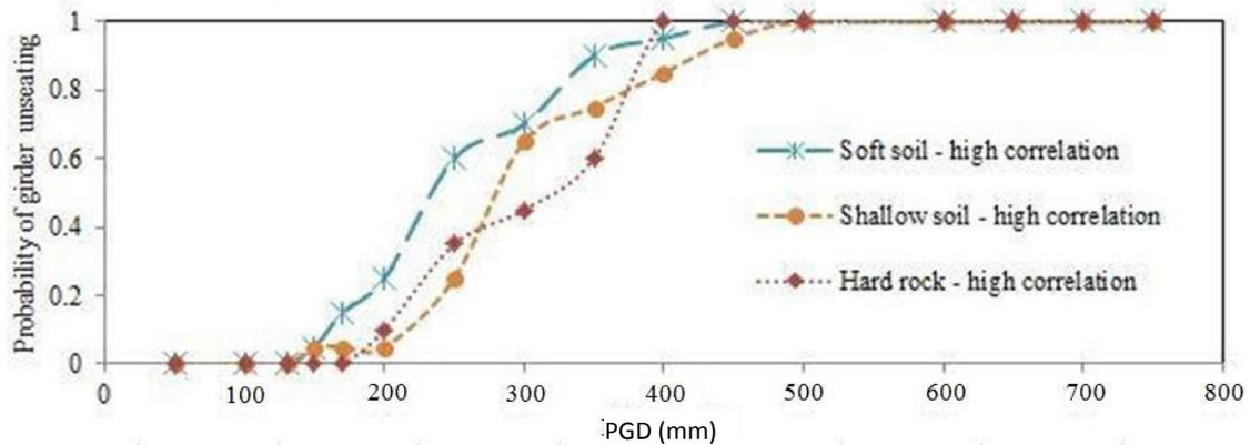
Fig. 6 Fragility curves for soft soil - highly correlated, shallow soil, and hard rock conditions based on the NZTA bridge manual requirements
