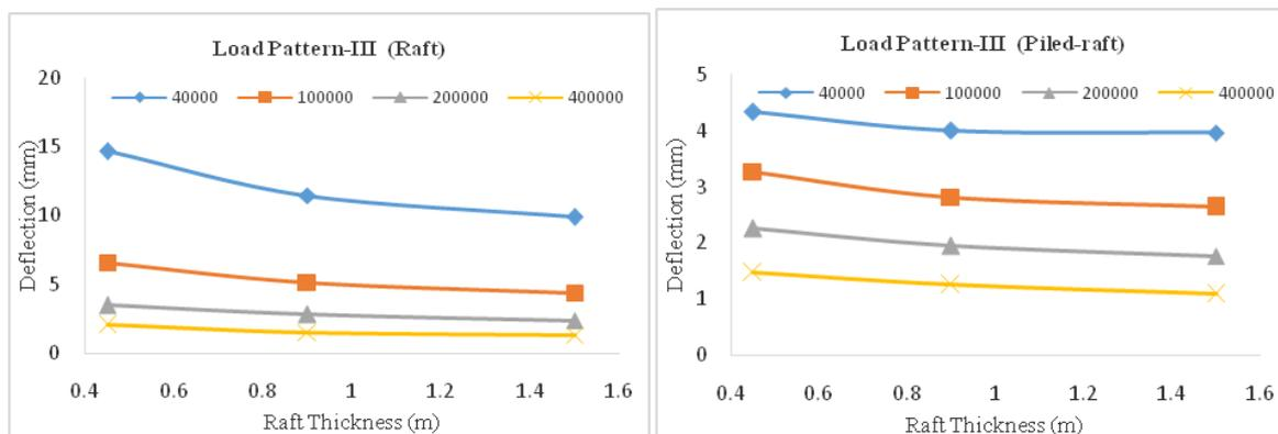
Fig. 11 Variation in maximum deflection with raft thickness in raft and piled raft for load pattern-III
