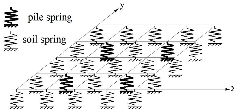
Fig. 2 Structural idealization for piled raft and supporting soil
