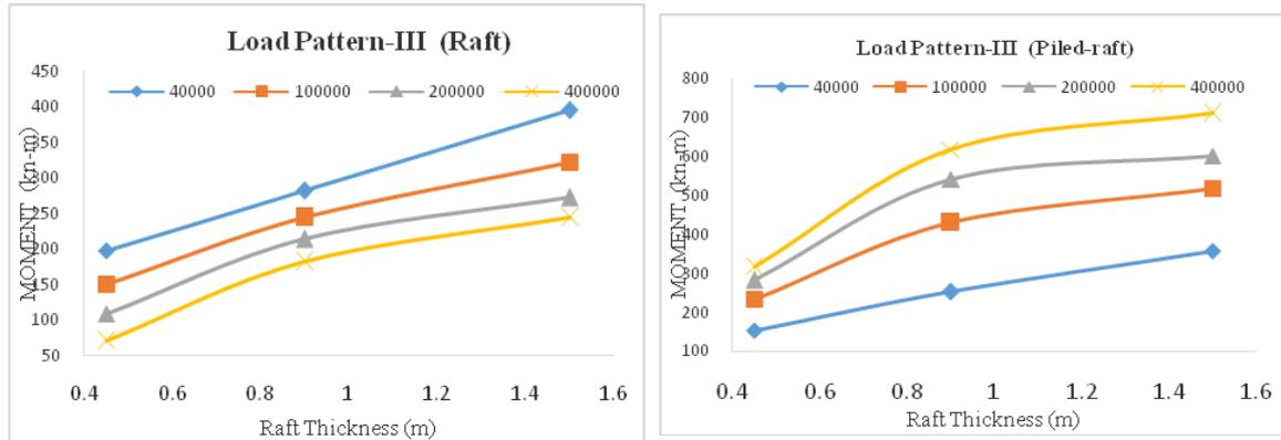
Fig. 12 Variations of maximum moment with raft thickness in raft and piled raft for load pattern-III
