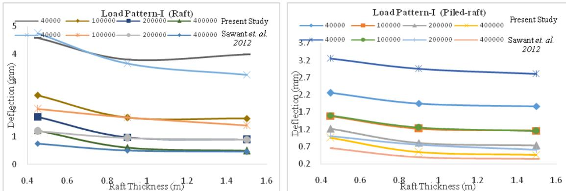
Fig. 7 Variation in maximum deflection in raft and piled raft with raft thickness for load pattern-I
