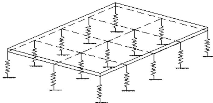
Fig. 1 Structural idealization with raft and supporting soil
