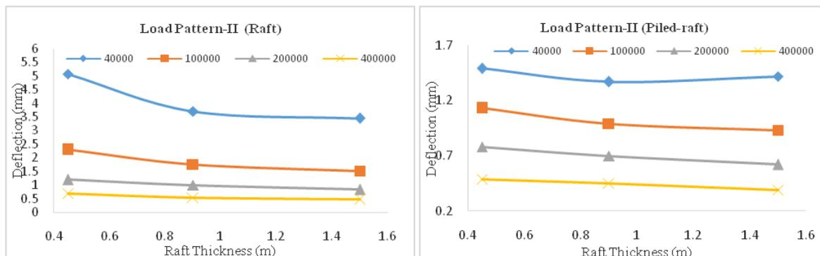
Fig. 9 Variation in maximum deflection with raft thickness in raft and piled raft for load pattern-II
