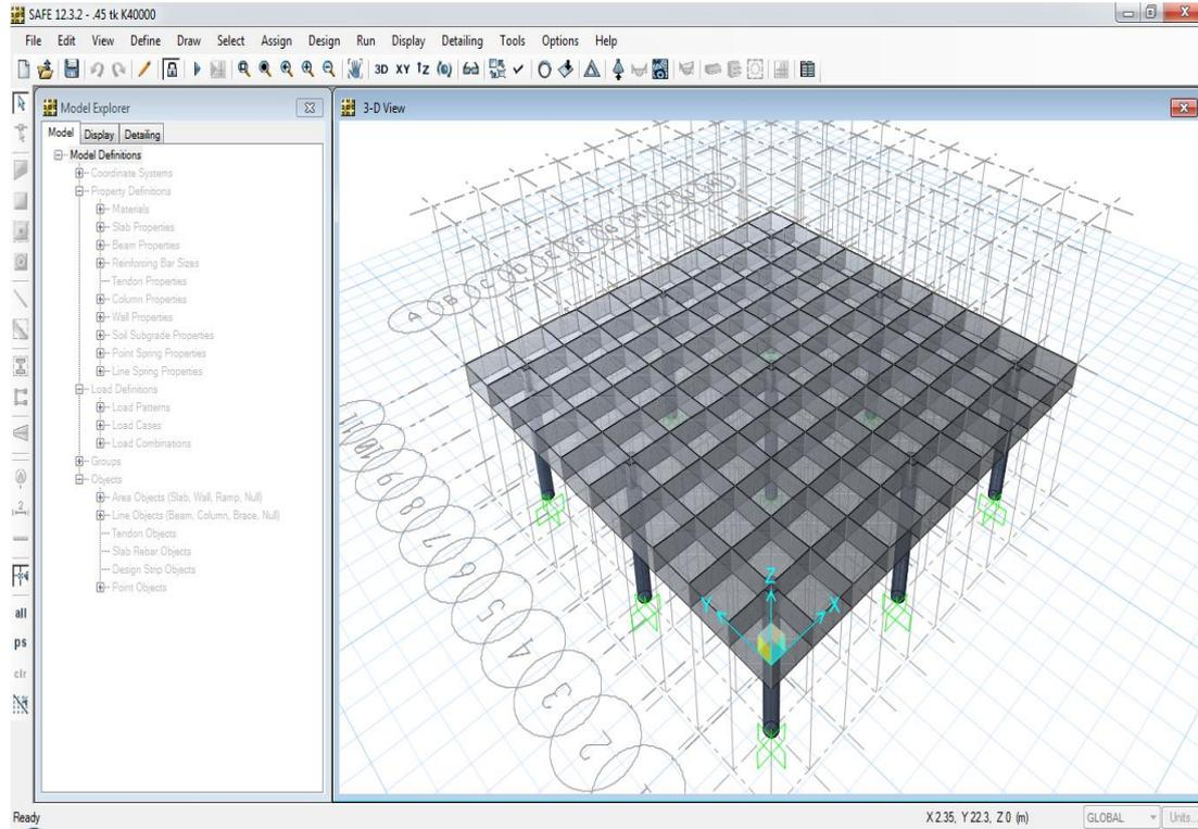
Fig. 6 Generalized F.E. model using SAFE for load pattern under consideration
