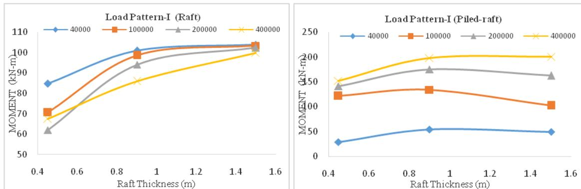
Fig. 8 Variation in maximum moment with raft thickness in raft and piled raft for load pattern-I
