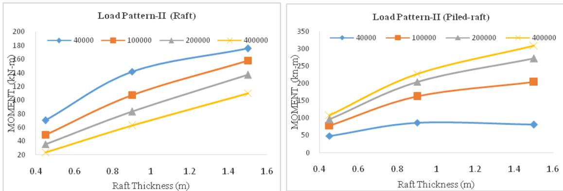
Fig. 10 Variations of maximum moment with raft thickness for raft and piled raft for load pattern-II
