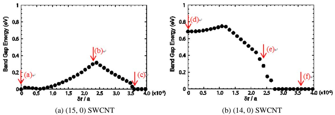
Fig. 3 Change in band gap energy under radial corrugation
