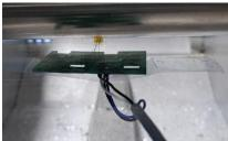
Fig. 1 Experimental set-up with the detail of strain gauges for indirect displacement measurement
