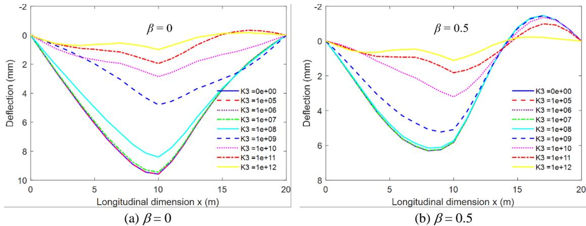
Fig. 8 Deflected shapes of longitudinal centerline when a load is at the center for various values of nonlinear stiffness
