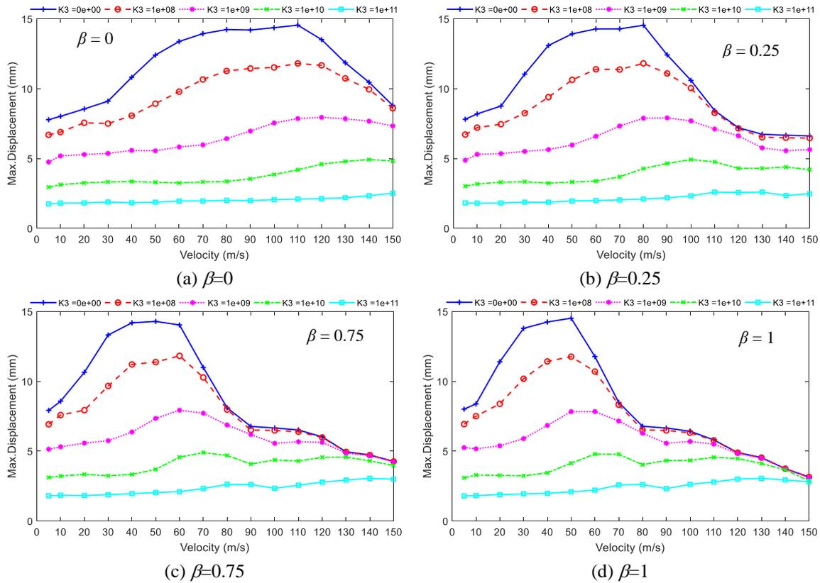
Fig. 12 Effects of the varying load velocities and nonlinear stiffness on max displacement
