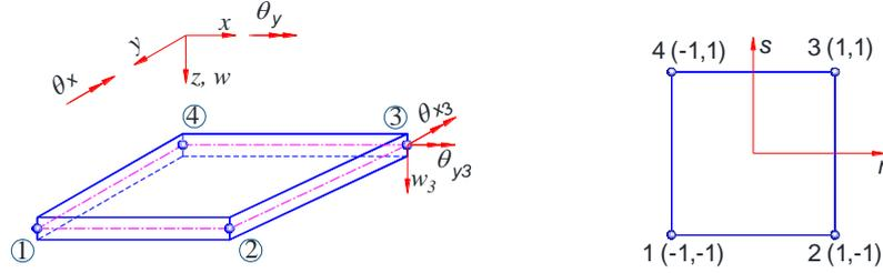
Fig. 4 Quadrilateral four-node elements,  $Q4$ : (a) in global coordinates; (b) in natural coordinates
