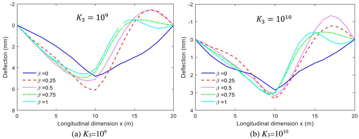
Fig. 11 Deflected shapes of longitudinal centerline when a load is at center for various foundation mass
