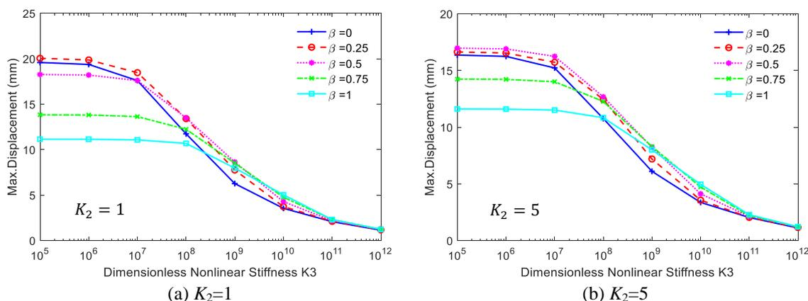
Fig. 15 Effects shear stiffness on max displacement for various nonlinear stiffness and foundation mass where  $K_1 = 50$ ,  $c_f = 100 \text{ Ns/m}^3$
