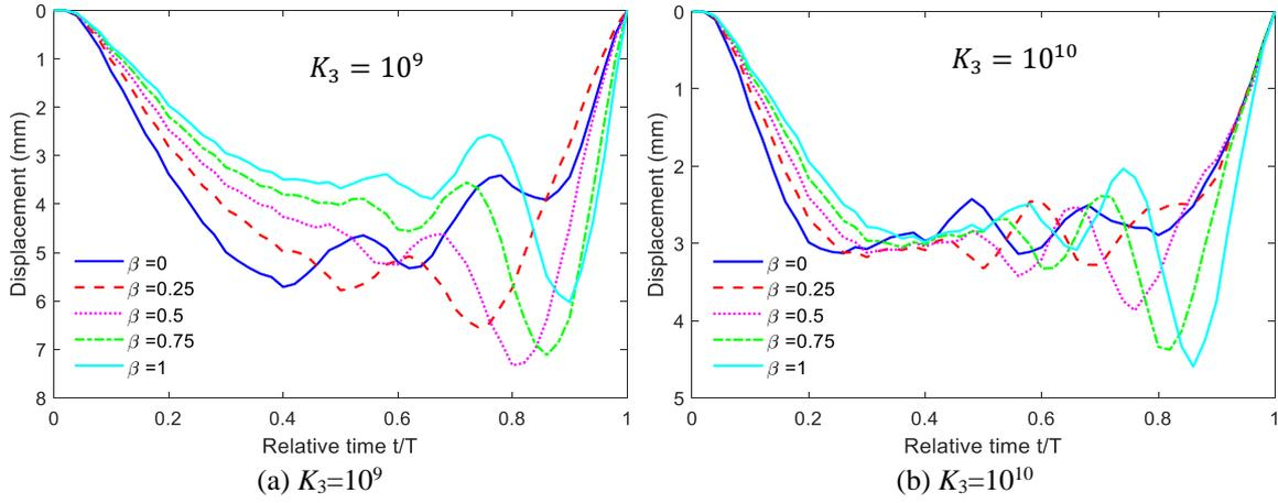
Fig. 10 Vertical displacement under moving load for various foundation mass
