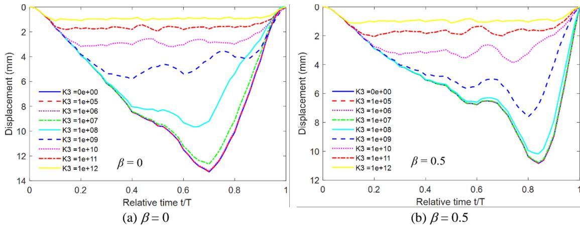
Fig. 7 Vertical displacement under moving load for various values of nonlinear stiffness
