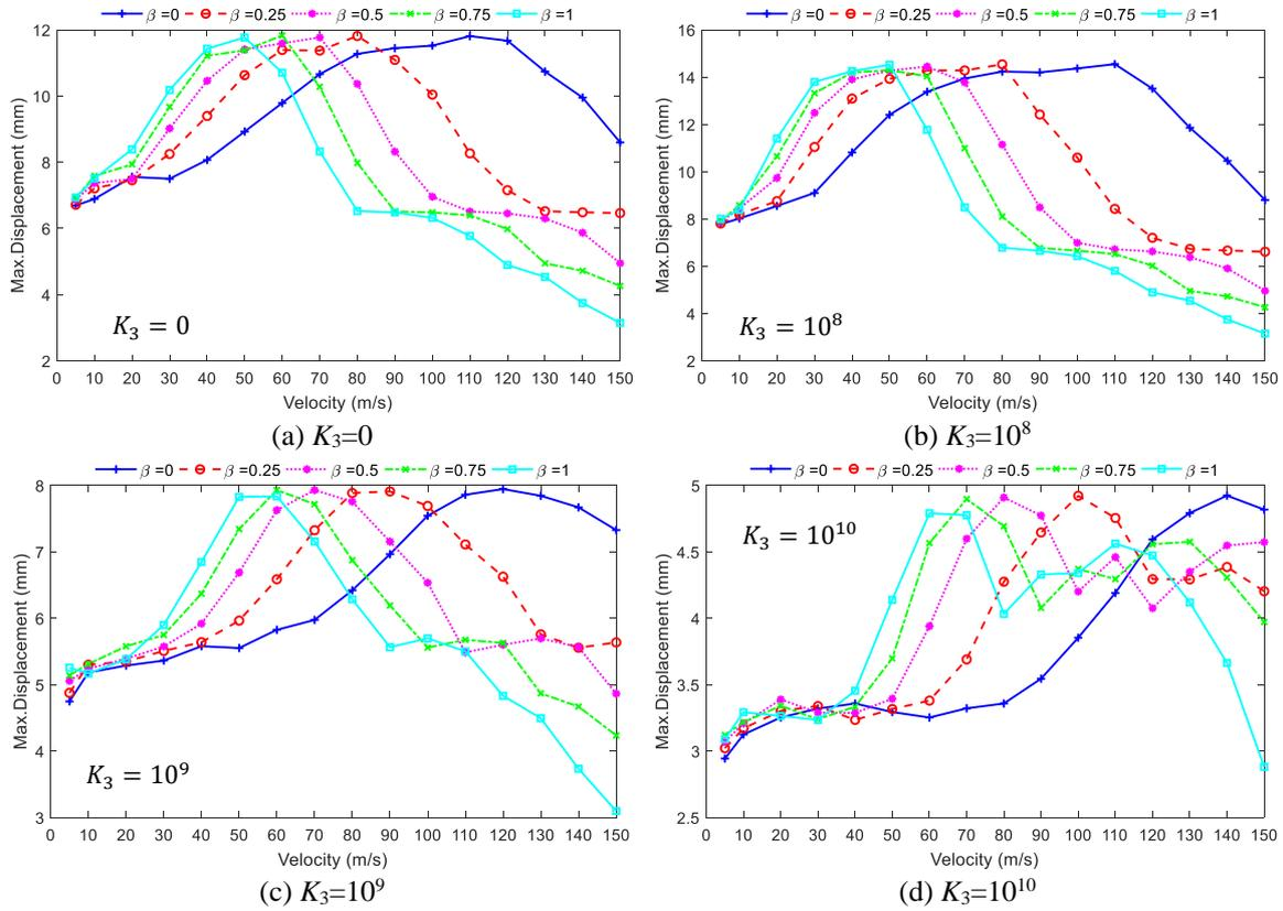
Fig. 13 Effects of the varying load velocities and foundation mass on max displacement
