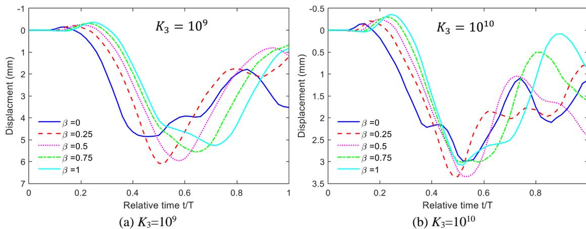
Fig. 9 The vertical displacement of central point of plate for various foundation mass
