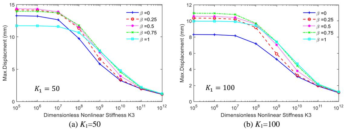
Fig. 14 Effects of linear stiffness on max displacement for various nonlinear stiffness and foundation mass where  $K_2 = 10$ ,  $c_f = 100$  Ns/m<sup>3</sup>
