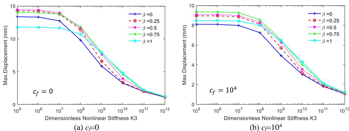
Fig. 16 Effects viscous damping of foundation on max displacement for various nonlinear stiffness and foundation mass where  $K_1 = 50$ ,  $K_2 = 10$
