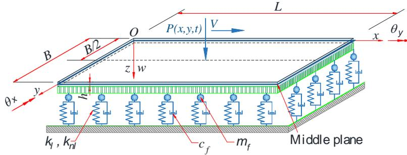
Fig. 3 Model of Mindlin plate on nonlinear dynamic foundation under moving load
