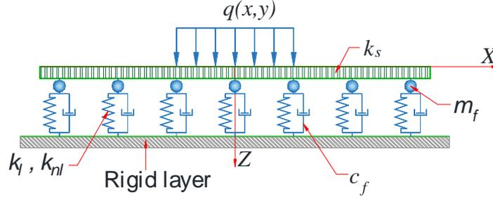
Fig. 1 The dynamic foundation model
