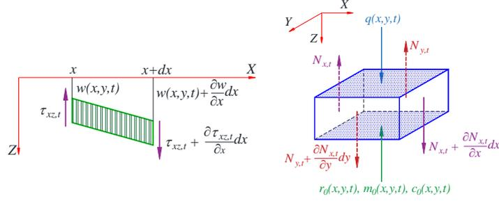
Fig. 2 Dynamic equilibrium on the shear layer: (a) stresses; (b) forces acting
