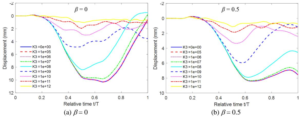
Fig. 6 The displacement of the central point of plate for various values of nonlinear stiffness
