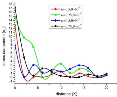
Fig. 6 Variation of stress component  $\sigma_{11}$  with distance  $x$  (uniformly distributed force)
