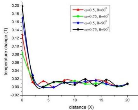
Fig. 15 Variation of temperature change  $T$  with distance  $x$  (linearly distributed force)
