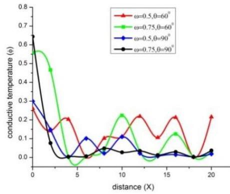
Fig. 7 Variation of conductive temperature  $\phi$  with distance  $x$  (uniformly distributed force)
