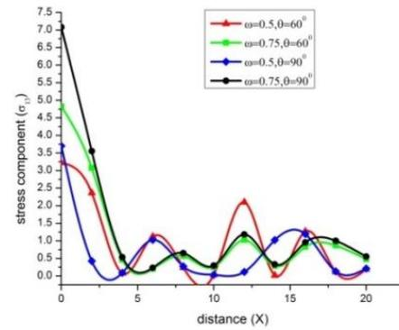
Fig. 12 Variation of stress  $\sigma_{31}$  with distance  $x$  (linearly distributed force)
