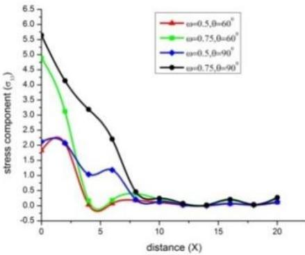
Fig. 11 Variation of stress  $\sigma_{33}$  with distance  $x$  (uniformly distributed force)
