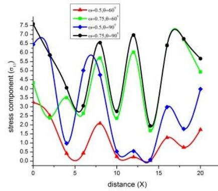
Fig. 5 Variation of stress component  $\sigma_{13}$  with distance  $x$  (uniformly distributed force)
