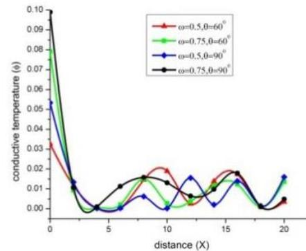
Fig. 14 Variation of conductive temperature  $\phi$  with distance  $x$  (linearly distributed force)
