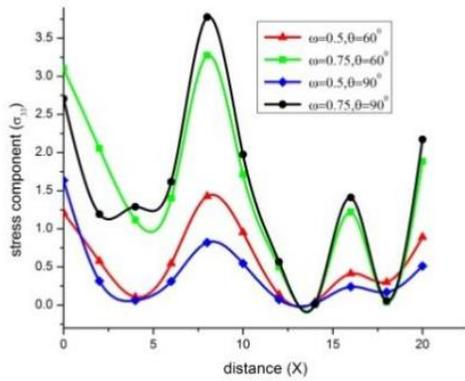
Fig. 4 Variation of stress component  $\sigma_{33}$  with distance  $x$  (uniformly distributed force)
