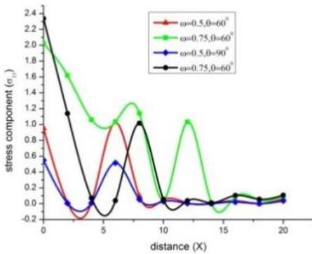
Fig. 13 Variation of stress component  $\sigma_{11}$  with distance  $x$  (linearly distributed force)
