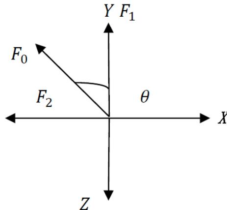
Fig. 1 Inclined load on an orthotropic thermoelastic solid
