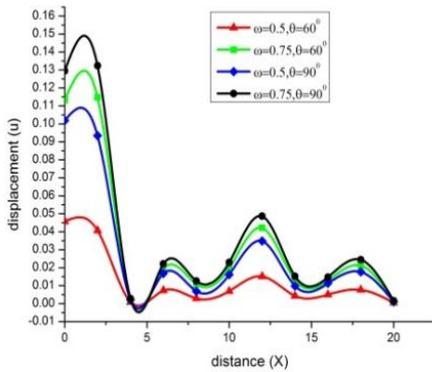
Fig. 9 Variation of displacement  $u$  with distance  $x$  (linearly distributed force)
