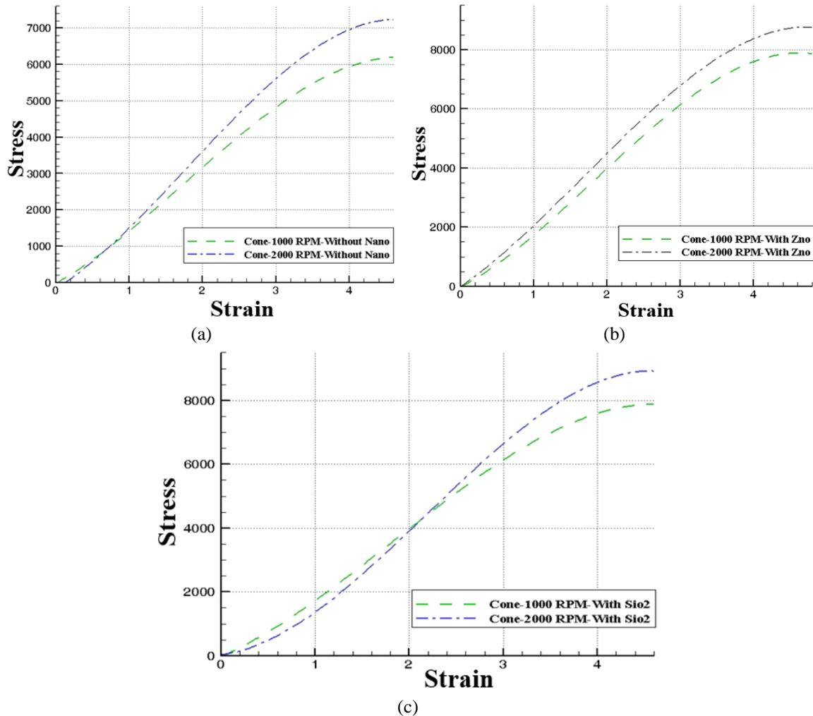
Fig. 7 Samples with Cone surface without nanoparticles under bending test, (b) samples with Cone surface with ZnO nanoparticles under bending test, (c) samples with Cone surface with SiO<sub>2</sub> nanoparticles under bending test
