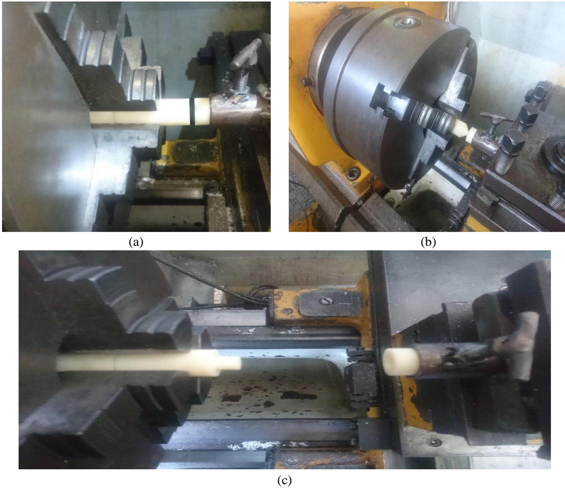
Fig. 2 (a) Flat surface ready to welding, (b) Cone surface ready to welding, (c) Step surface ready to welding
