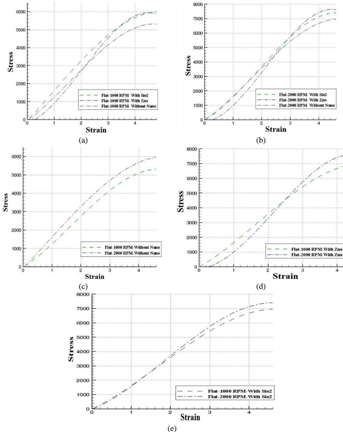
Fig. 6 (a) Shows the machining parameters in terms of the different rotation speeds in Flat surfaces, (b) shows the machining parameters in terms of the different rotation speeds in Flat surfaces, (c) samples with Flat surfaces without nanoparticles under bending test, (d) samples with Flat surface with Zn nanoparticles under bending test, (e) samples with Flat surface with SiO<sub>2</sub> nanoparticles under bending test
