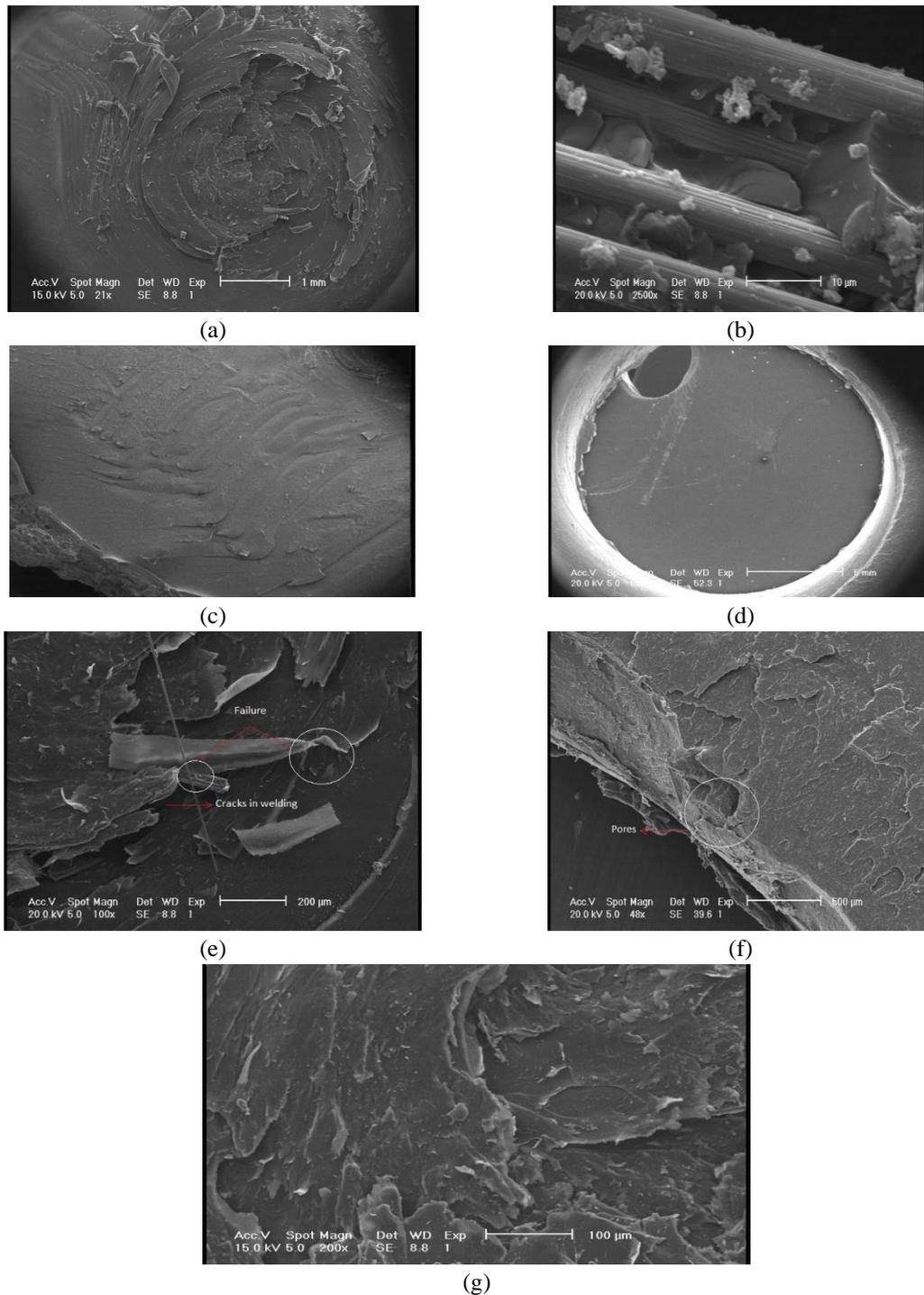
Fig. 10 (a) SEM shot on the welding area (b) Presence of Nanoparticles on welding area, (c) shows the SEM shot of ledge area, (d) shows the SEM shot of groove area, (e) shows the SEM shot of groove area, (f) shows the SEM shot of micro cracks, and sample failure on welding area, (g) shows the SEM shot of Pores on welding area
