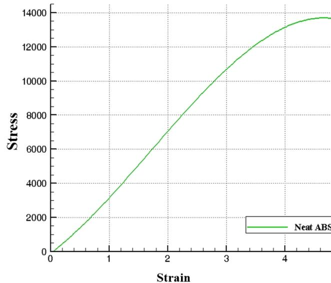
Fig. 5 Pure ABS bending test result
