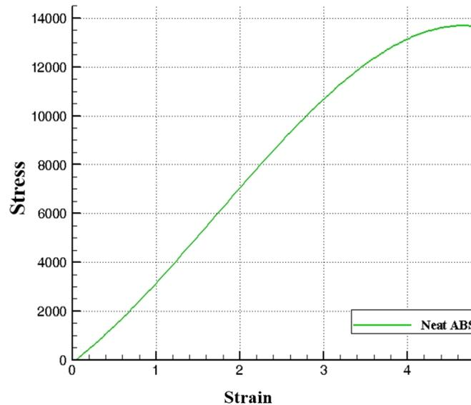
Fig. 5 Pure ABS bending test result
