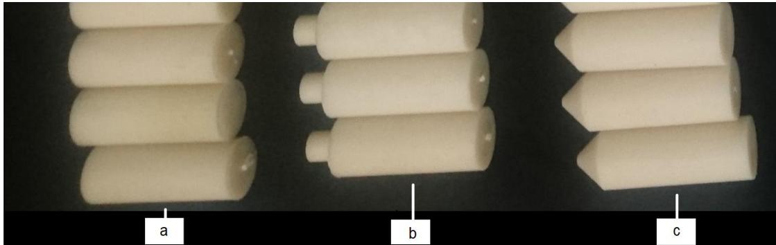
Fig. 1 Flat surface (a) Step surface (b) Cone surface (c)
