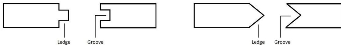
Fig. 1.1 Shape of the flat and cone surface
