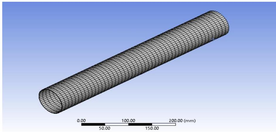
Fig. 8 The meshing of the optimum boundary geometry
