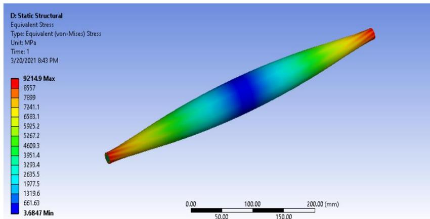
Fig. 11 Stress under twisting moment for a solid shaft of weight 0.09318 Kg
