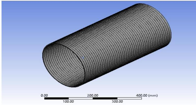
Fig. 2 The meshing of the Upper boundary geometry
