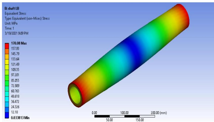
Fig. 7 Stress under twisting moment
