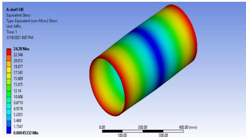
Fig. 4 Stress under twisting moment
