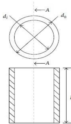
Fig. 1 Hollow shaft
