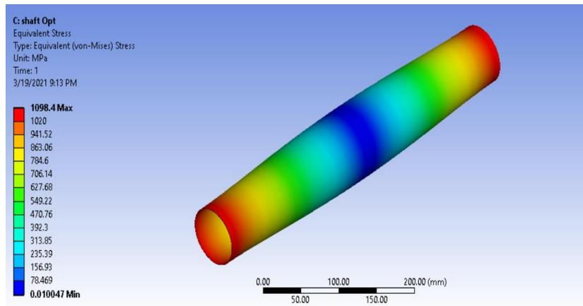
Fig. 10 Stress under twisting moment
