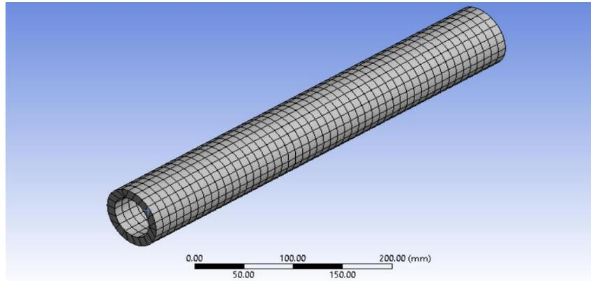
Fig. 5 The meshing of the lower boundary geometry
