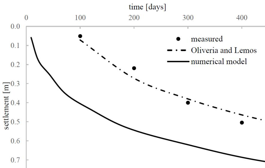
Fig. 10 Comparison of consolidation curves for first 450 days
