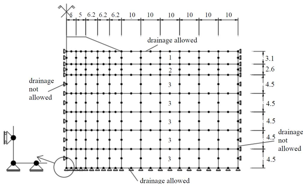
Fig. 8 Numerical model of embankment near the city of Boston
