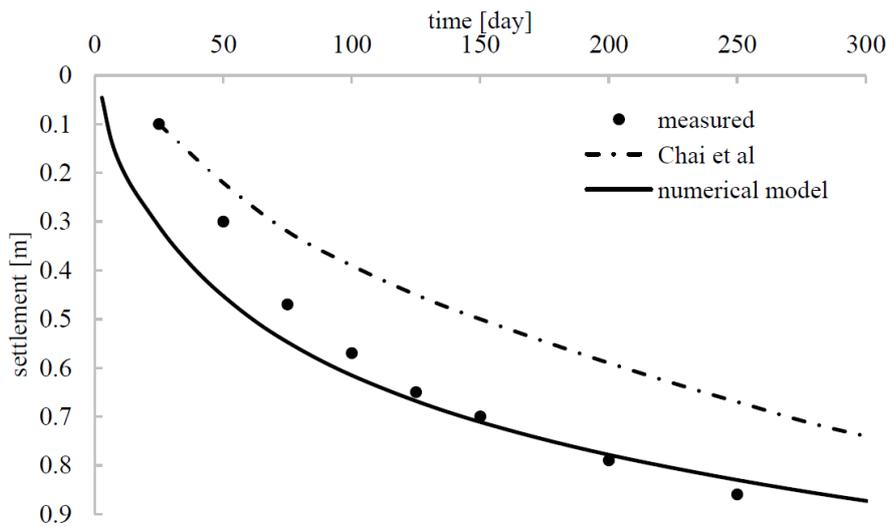
Fig. 7 Comparison of consolidation curves for first 300 days
