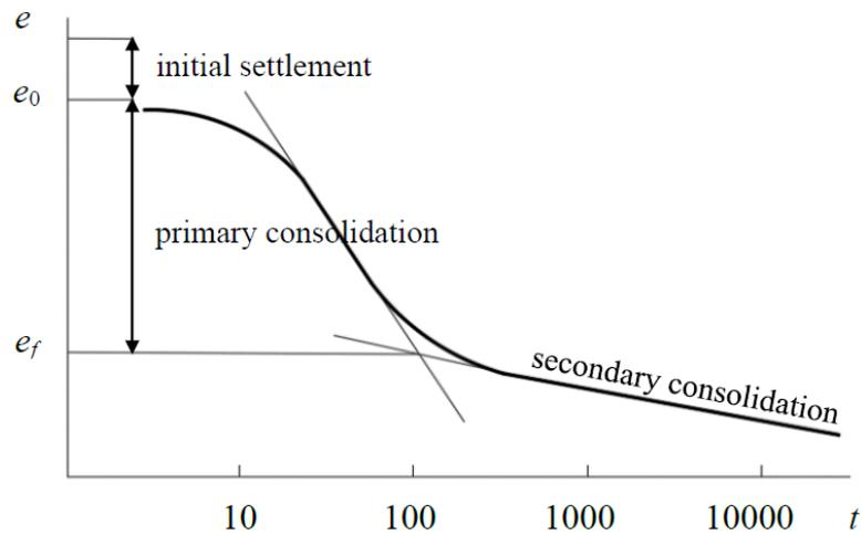
Fig. 1 Three stages of embankment total settlement (Maksimović 2008)
