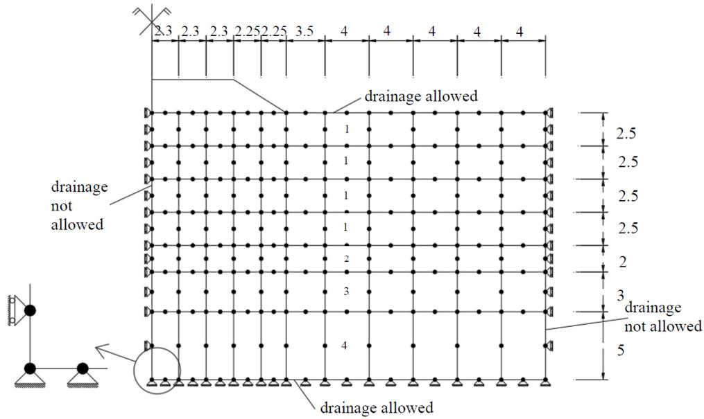
Fig. 5 Numerical model of embankment near the city of Saga
