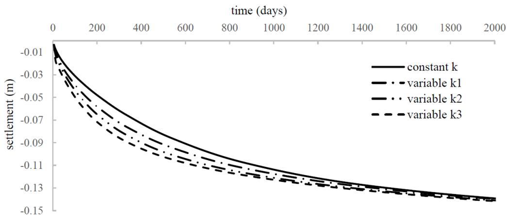
Fig. 4 Computed consolidation curves for the constant and strain-dependent coefficient of permeability
