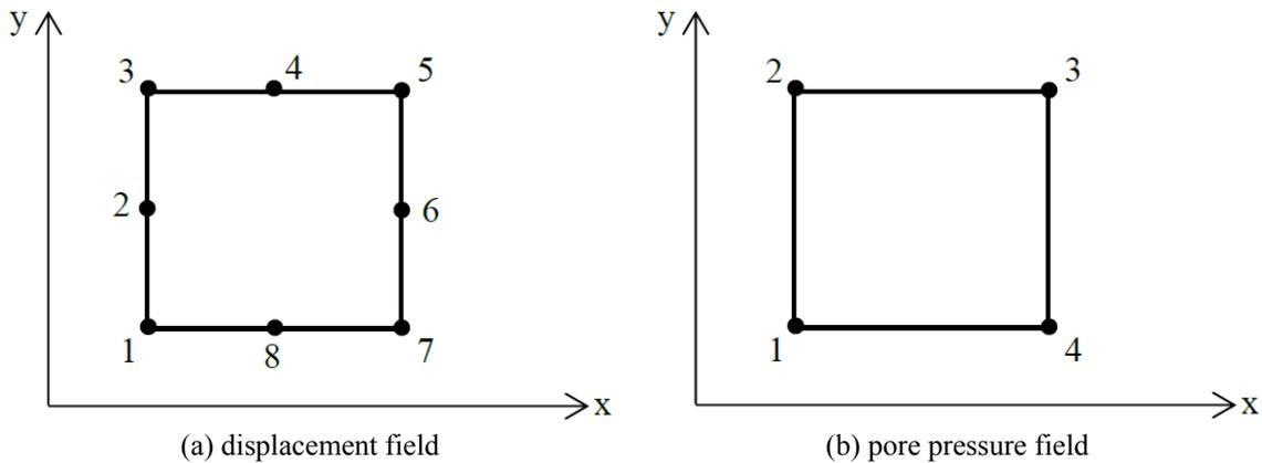
Fig. 3 Finite element approximations of unknown fields
