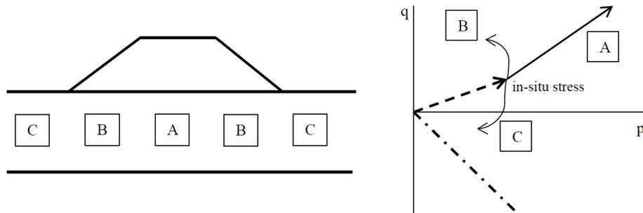
Fig. 2 Zones in soil under the embankment with different strain states
