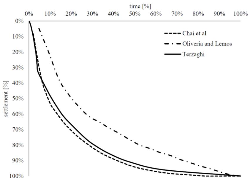
Fig. 11 Comparison of measured consolidation curves with Terzaghi's theoretical consolidation curve
