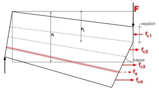
Fig. 4 Schematic representation of the layered beam model in three-point bending test
