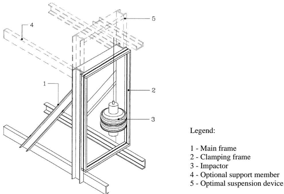
Fig. 2 Test setup for soft body impact according to HR EN 12600:2006 (EN 12600:2002)
