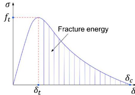
Fig. 6 A Typical stress-displacement curve (Wang *et al.* 2017)
