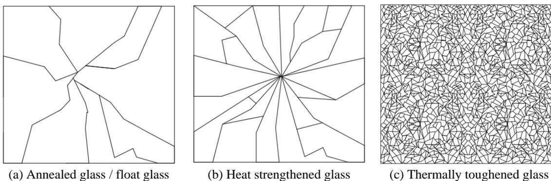
Fig. 1 Breakage pattern for each type of glass
