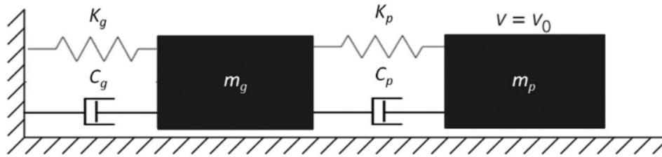
Fig. 4 Two degree of freedom model for simulation pendulum - glass contact during impact (Parra *et al.* 2019)
