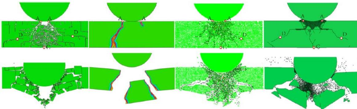
Fig. 7 Evolution of crack pattern for different calculation methods (from left to right FEM, XFEM, DEM and FEM/DEM respectively) (Wang *et al.* 2017)
