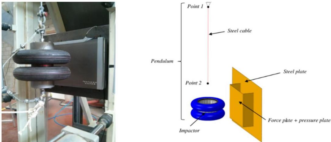
Fig. 5 Test setup with pendulum and pressure plate, simulation of pendulum test (Pelfrene *et al.* (2016))
