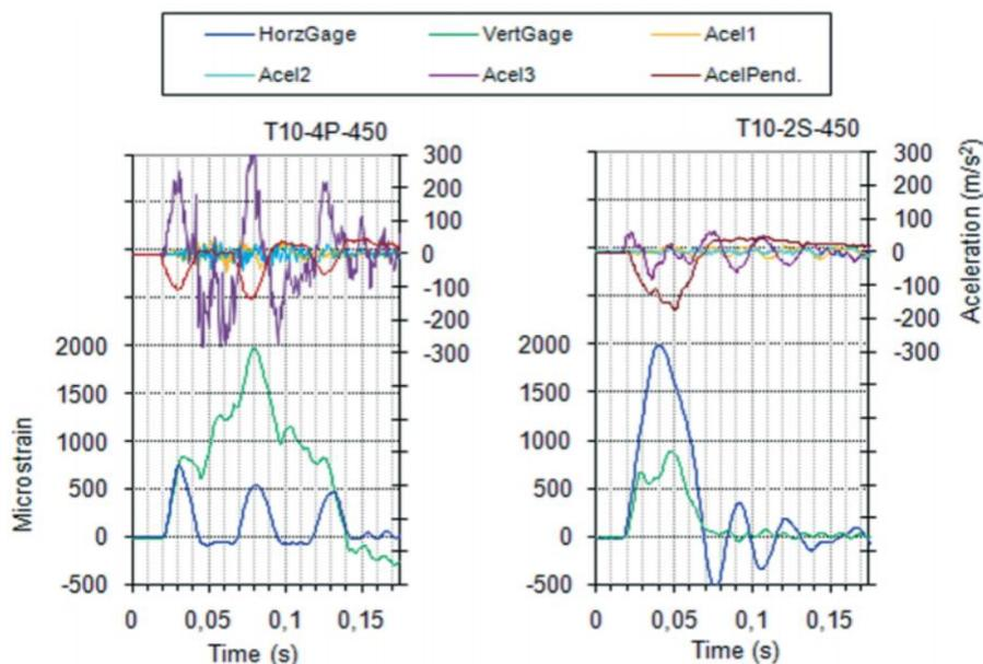
Fig. 3 Experimental results from pendulum impact test on four point supported (4P) and two sides (2S) supported glass panel, for same drop height (450 mm) (Pacios *et al.* 2011)
