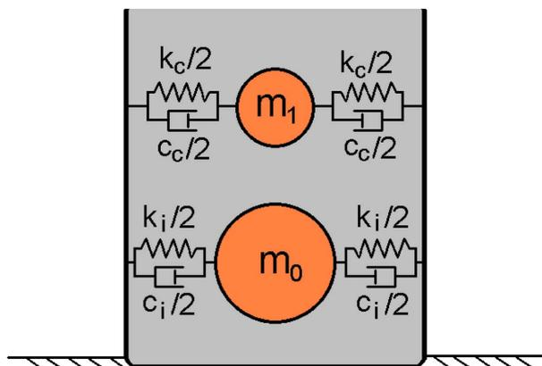
Fig. 2 Spring-mounted masses analogy for storage tanks
