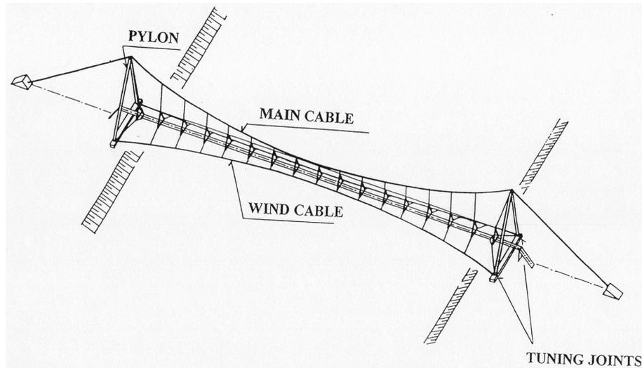
Fig. 1 Slender wood bridge with TVC-equipment
