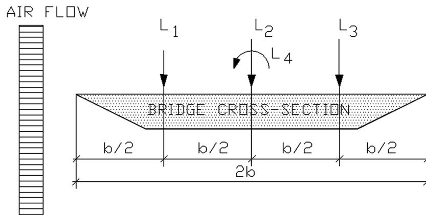
Fig. 2 Aeroelastic forces on the bridge
