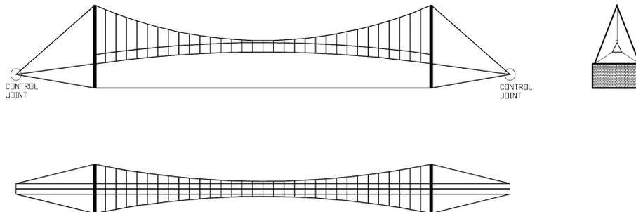
Fig. 5 Geometry of the wood bridge studied
