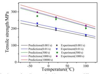
Fig. 2 The change of tensile strength with temperature at different strain rates
