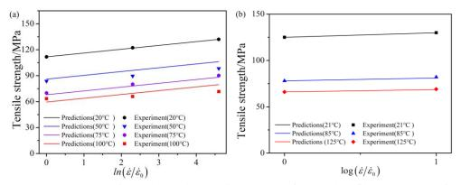
Fig. 3 Temperature and strain rate dependent tensile strength of short glass fiber/PA6 composites: (a) 33% vol fiber (The experimental data are quoted from Wang *et al.* (2002)) (b) 35% vol fiber (The experimental data are quoted from Mortazavian and Fatemi (2017))
