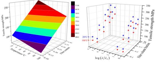
Fig. 5 The effect of fiber content on tensile strength
