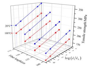
Fig. 6 The effect of average fiber length on tensile strength
