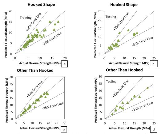
Fig. 5 Comparison between predicted and actual values for Flexural Strength on the Basis of Shape by GP technique
