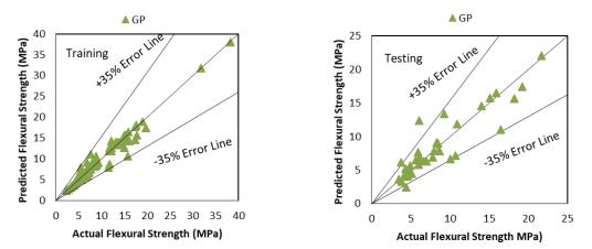
Fig. 3 Agreement plot between observed and predicted flexural strength of training and testing dataset by GP technique
