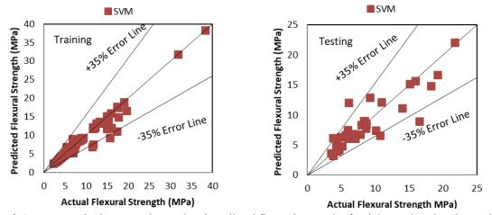
Fig. 2 Agreement plot between observed and predicted flexural strength of training and testing dataset by SVM technique
