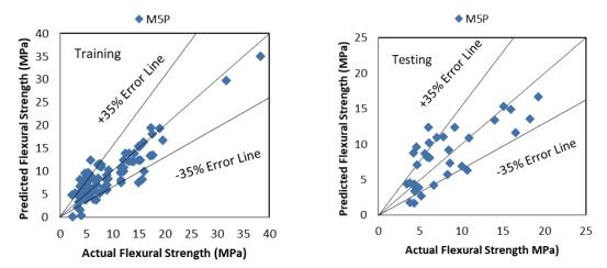
Fig. 1 Agreement plot between observed and predicted flexural strength of training and testing dataset by M5P technique
