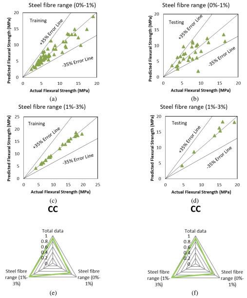
Fig. 7 Comparison between predicted and actual values for flexural strength on the basis of steel fibre percentage by GP technique
