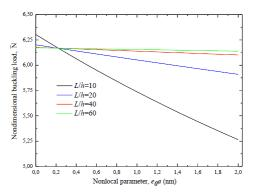
Fig. 5 Effect of nonlocal parameter on nondimensional buckling load for k = 1
