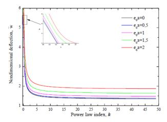
Fig. 6 Variation of the nondimensional deflection of S-S FGM nanobeam with material graduation and for different scale parameter rises (L/h = 10)
