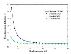
Fig. 2 Effect of the length to thickness ratio on dimensionless deflection for uniform load for k = 1,  $e_0 a = 1$  nm
