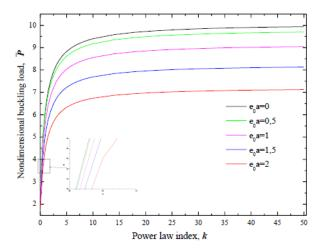
Fig. 7 Variation of the nondimensional buckling load of S-S FGM nanobeam with material graduation and for different scale parameter rises (L/h = 10)
