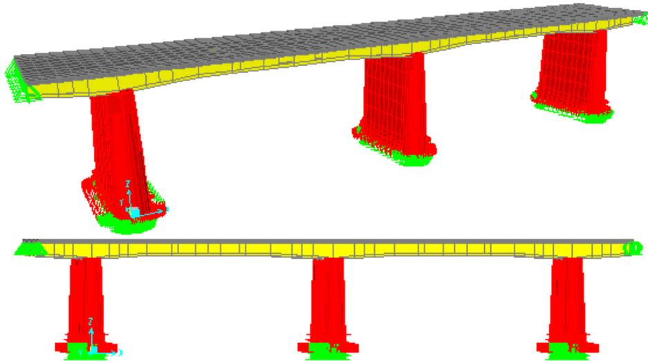
Fig. 2 Three dimensional initial finite element model of the bridge beam
