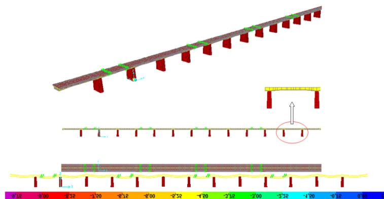
Fig. 10 The maximum vertical displacements of the bridge before model updating under dead load
