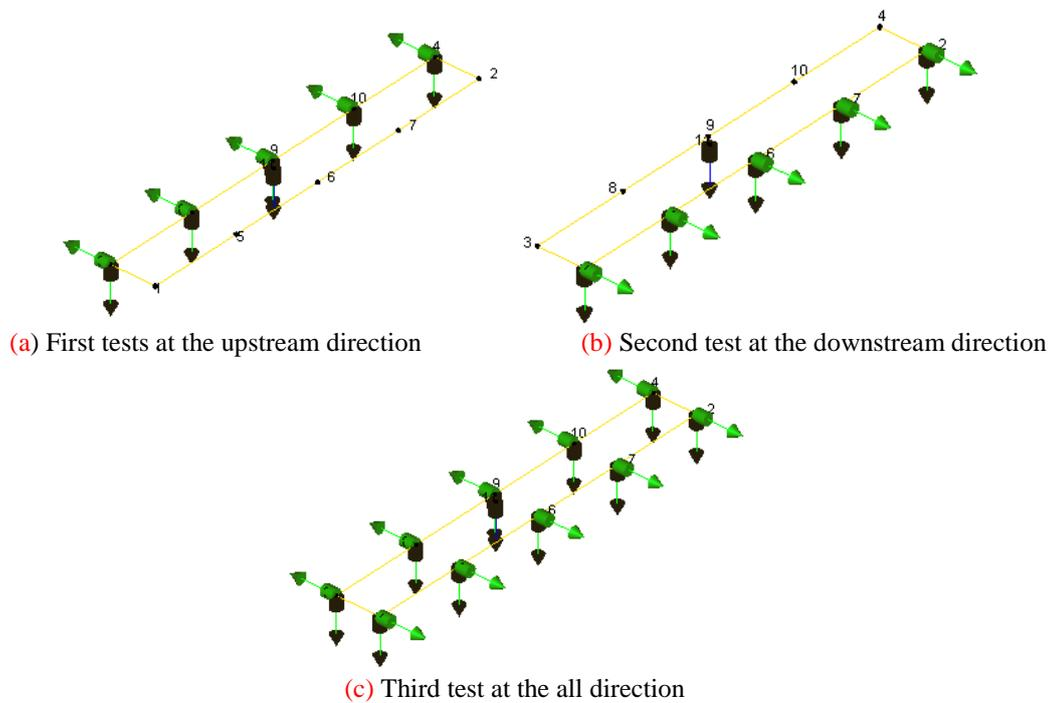
Fig. 5 The accelerometer locations for each experimental measurement
