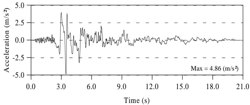
Fig. 14 Time history of ground motion acceleration of 1992 Erzincan earthquake
