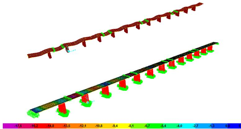
Fig. 21 The maximum vertical displacements of the bridge after model updating under dynamic load
