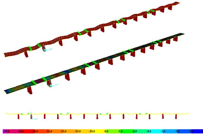
Fig. 12 The maximum vertical displacements of the bridge before model updating under increased live load
