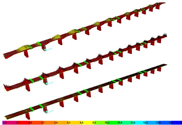
Fig. 13 Distribution of maximum internal forces and stresses before model updating under increased live load
