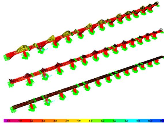
Fig. 20 Distribution of maximum internal forces and stresses after model updating under increased live load
