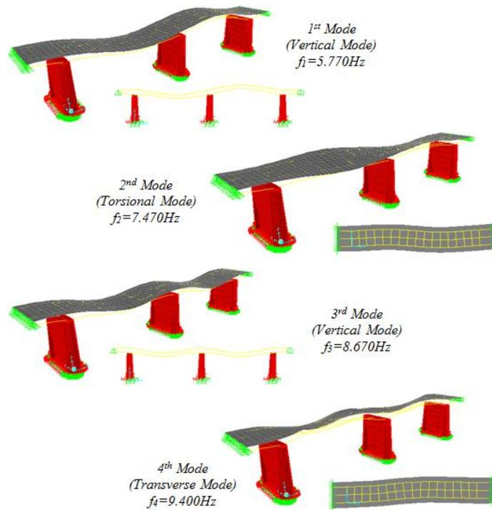
Fig. 3 Analytically identified the first four mode shapes
