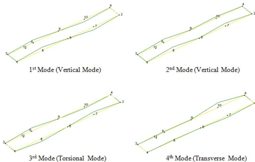
Fig. 7 Experimentally identified first four mode shapes
