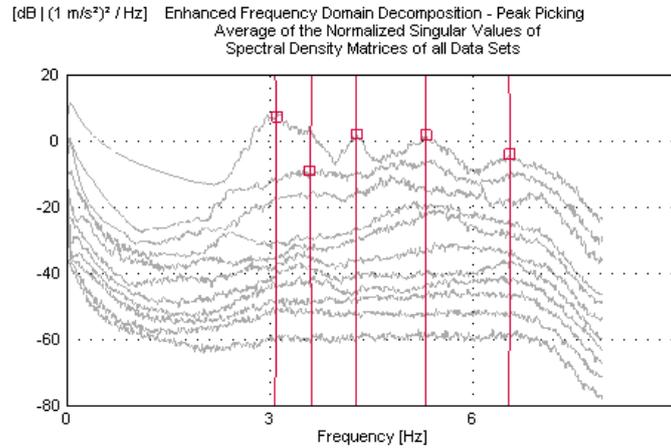
Fig. 6 Singular values of spectral density matrices
