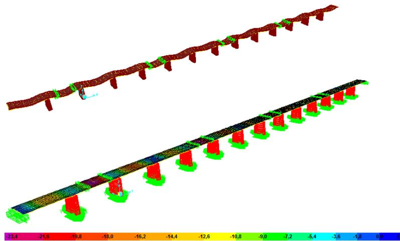
Fig. 15 The maximum vertical displacements of the bridge before model updating under dynamic load
