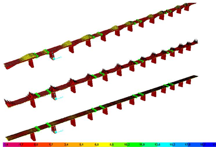
Fig. 16 Distribution of maximum internal forces and stresses before model updating under dynamic load
