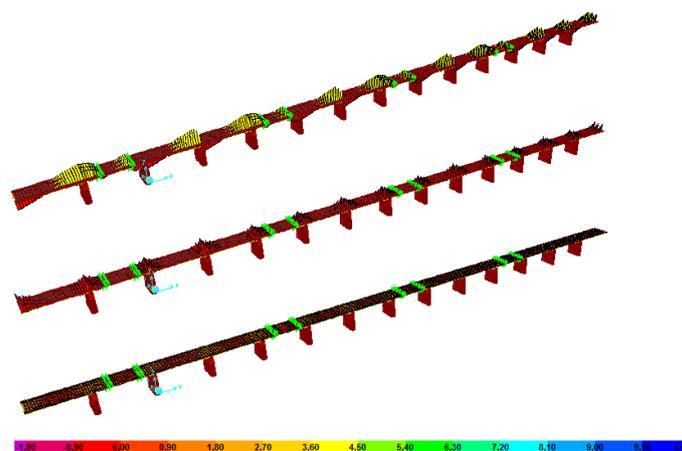
Fig. 11 Distribution of maximum internal forces and stresses before model updating under dead load
