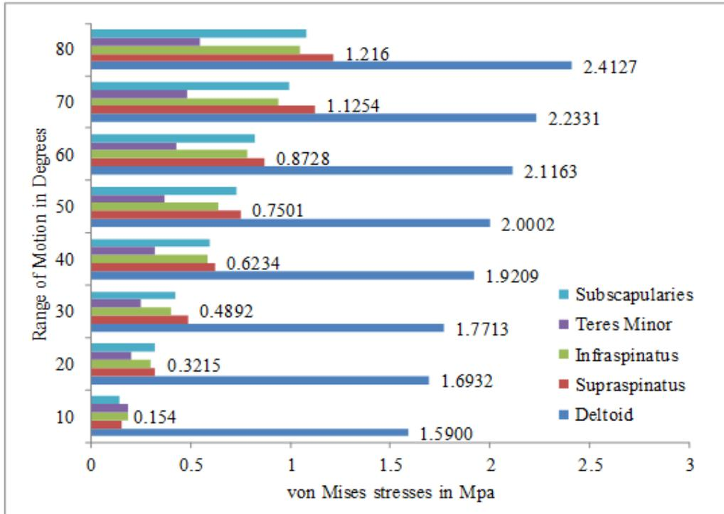
Fig. 8 von Mises stresses distribution during group muscle analysis for abduction arm movement
