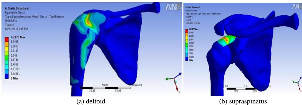
Fig. 9 von Mises stress distribution for individual muscle analysis
