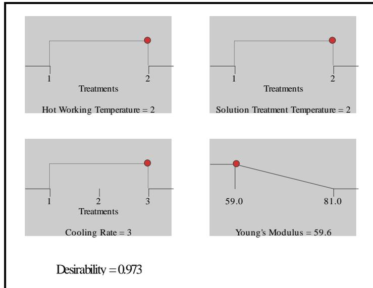
Fig. 6 Ramp function graph for Young's modulus after thermo-mechanical processing
