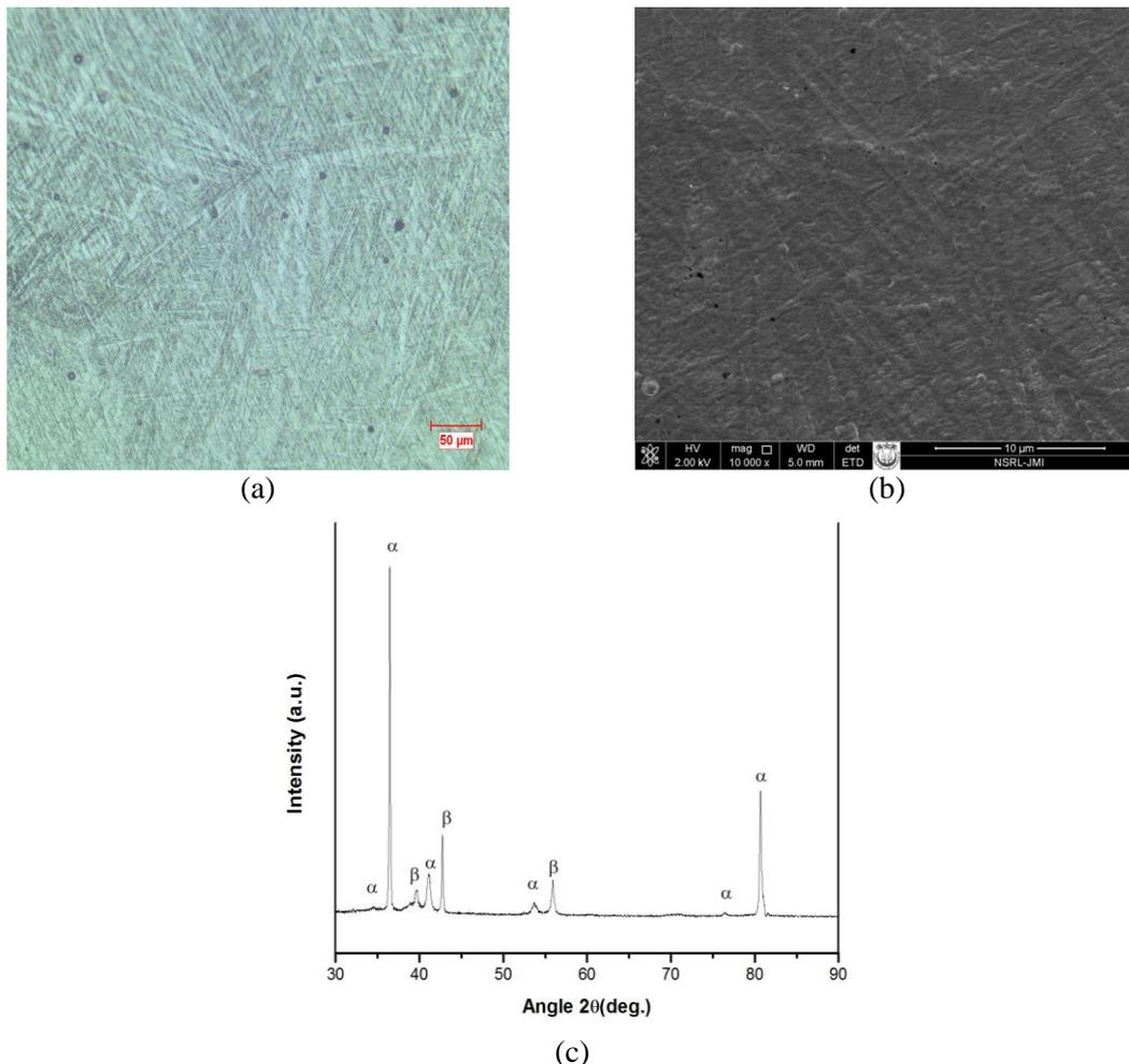
Fig. 2 Microstructure of as-cast TNZV alloy: (a) Optical Micrograph, (b) Scanning Electron Microstructure (SEM), (c) X-ray diffraction profiles
