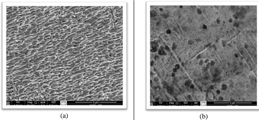
Fig. 5 Scanning electron microstructures (20000X) of the TNZV alloy (a) deformed at 850°C and solution treated at 650°C for 1h followed by AC, (b) deformed and solution treated at 850°C for 1h followed by WQ
