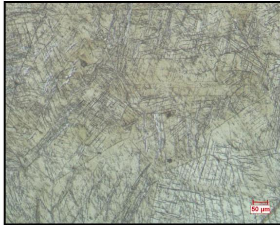
Fig. 3 Optical microstructures of the TNZV alloy deformed at 850°C and solution treated at 850°C for 1h followed by water quenching
