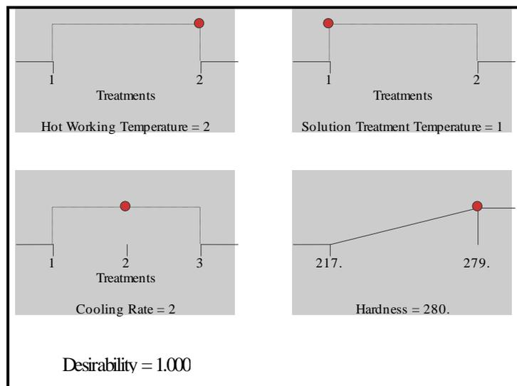
Fig. 4 Ramp function graph for micro-hardness after Thermo-mechanical processing
