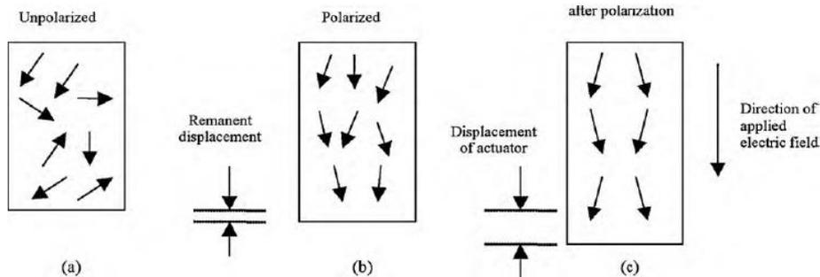
Fig. 6 Polarization process for a piezoelectric actuator (Devasia *et al.* 2007)
