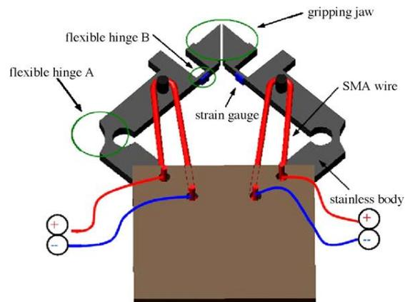
Fig. 14 Conceptual drawing of microgripper (Kyung *et al.* 2007)
