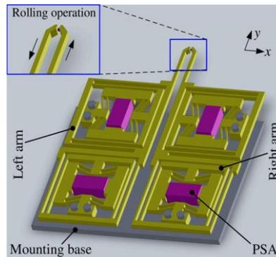
Fig. 10 A two-arm 2-DOF microgripper (Xu 2012)
