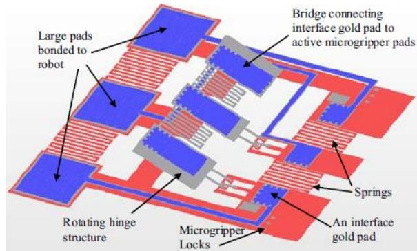
Fig. 12 3-D schematic drawing of the proposed interface (Anis *et al.* 2006)
