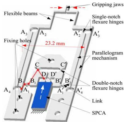
Fig. 8 3-D drawing of the MCM with an SPCA (Wang *et al.* 2011)
