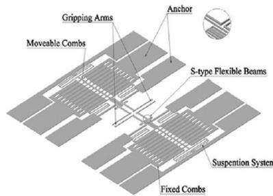
Fig. 4 An electrostatic microgripper design (Hamedi *et al.* 2012)
