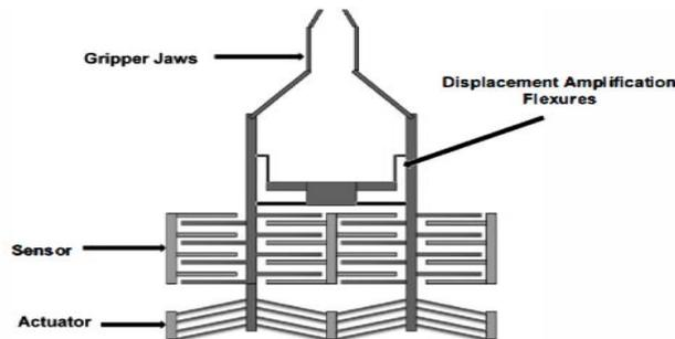
Fig. 5 Schematic diagram of electrothermal microgripper (Ali *et al.* 2011)
