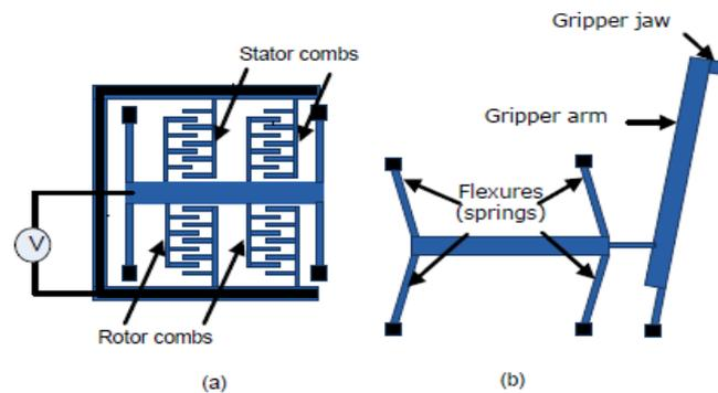
Fig. 2 (a) Voltage applied to actuator combs (b) Gripper arm bent due to force applied by the comb drives (Amjad *et al.* 2008)
