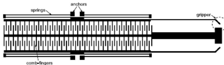
Fig. 1 Typical comb-drive based microgripper actuator (Varona *et al.* 2009)
