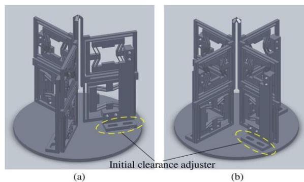
Fig. 11 (a) A three-arm and (b) a four-arm microgrippers (Xu 2012)
