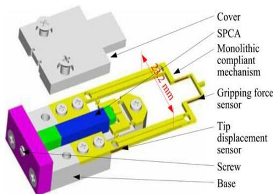
Fig. 7 Exploded 3-D drawing of the MCM based piezoelectric-driven microgripper (Wang *et al.* 2011)
