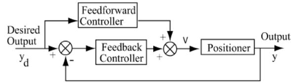
Fig. 16 Control scheme augmenting feedback with feedforward (Clayton *et al.* 2009)
