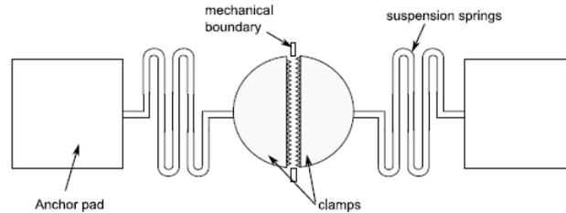
Fig. 3 A microgripper based on parallel-plate capacitance (Varona *et al.* 2009)
