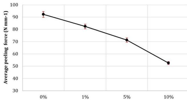
Fig. 7 Average peeling force versus the TiO<sub>2</sub> volume contents
