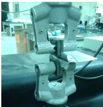
Fig. 2 Schematic illustration of the peeling test fixture
