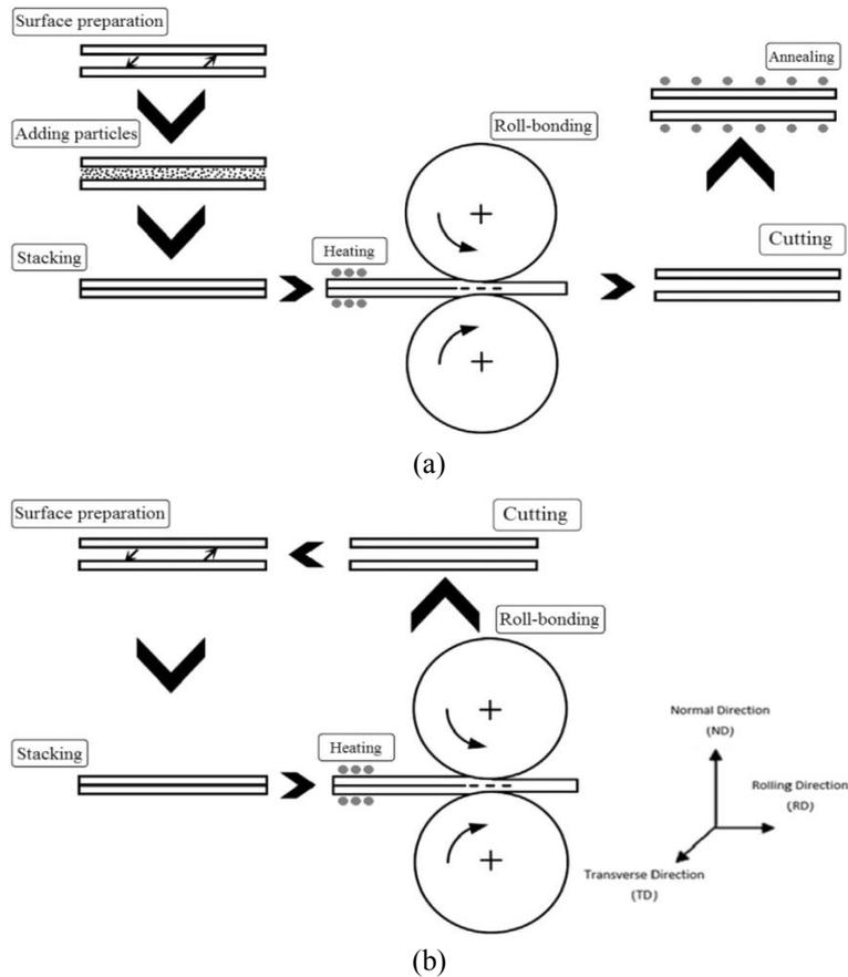
Fig. 1 Schematic illustration of the production process of Al/TiO<sub>2</sub> composite sheets (a) primary cycle (cycle#0) and (b) main cycles
