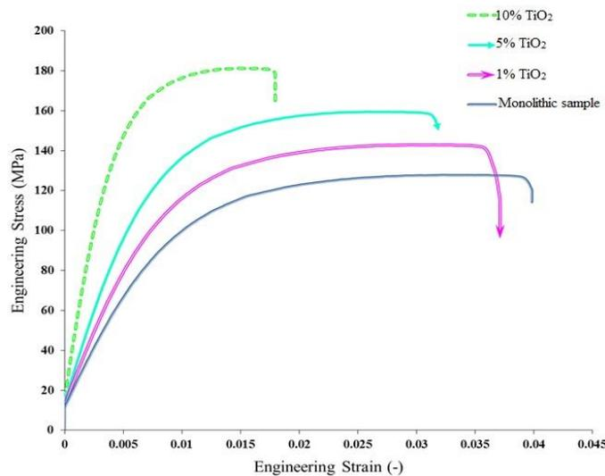
Fig. 3 Engineering stress-strain tensile test curves for AA1060/TiO<sub>2</sub> composites
