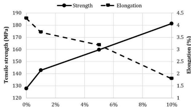
Fig. 4 Tensile strength and elongation of the Al/TiO<sub>2</sub> composites with the TiO<sub>2</sub> volume contents
