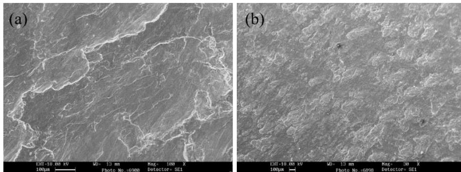
Fig. 8 SEM image of a peeled surface of samples with (a) 0%; and (b) 10% of TiO<sub>2</sub> particles volume contents
