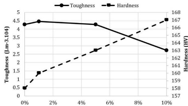
Fig. 5 Variations of toughness and hardness of composite samples with the TiO<sub>2</sub> volume percentages
