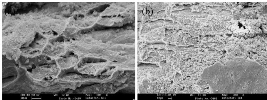
Fig. 6 Fracture surfaces after tensile test: (a) Al/1 vol%; and (b) Al/10 vol% TiO<sub>2</sub>
