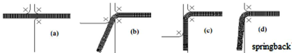
Fig. 2 Numerical simulation of folding process
