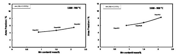
Fig. 6 The effect of Mn on the area fraction of MA at constant Nb (0.015%) after different heat cycles
