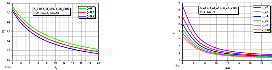
Fig. 7 Effect of Pasternak shear modulus parameter J_0 on dimensionless center deflection \bar{w} of FGM plates
