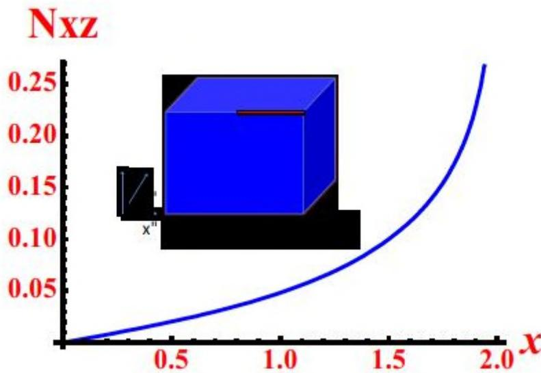
Fig. 5 The calculated demagnetization factor  $N_{xz}$  along the top edge of the sample.  $X=0$  corresponds to midpoint of edge and  $x=2$  to corner (see inset)
