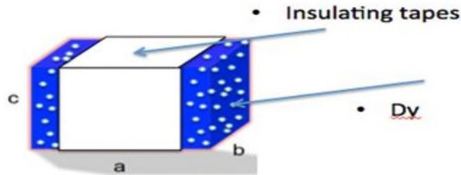
Fig. 1 Schematic of the N-38 Dy-free Neo magnet surfaces where Dy was sputter-coated onto the edges (other areas were masked).
