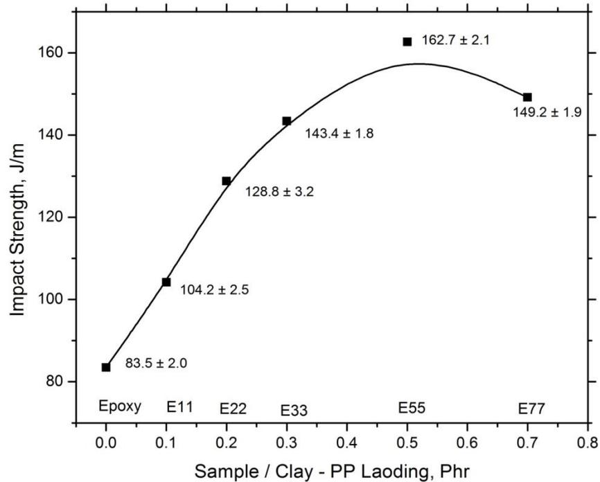
Fig. 1 Impact strengths of epoxy-PP short fibers-clay composites
