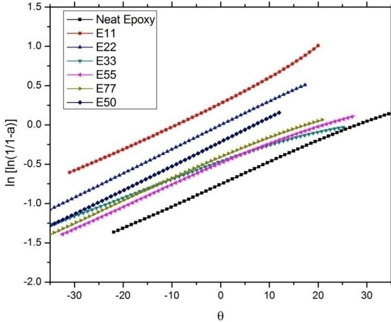
Fig. 7 Horowitz-Metzger kinetic plot to find  $E_a$  of epoxy-PP short fibers-clay composites
