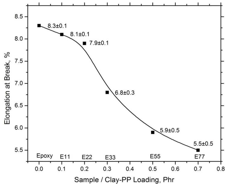
Fig. 5 Elongation at break of epoxy-PP short fibers -clay composites
