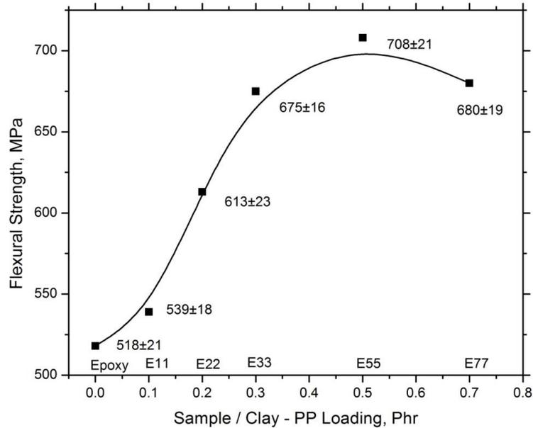
Fig. 4 Flexural strength of epoxy-PP short fibers -clay composites
