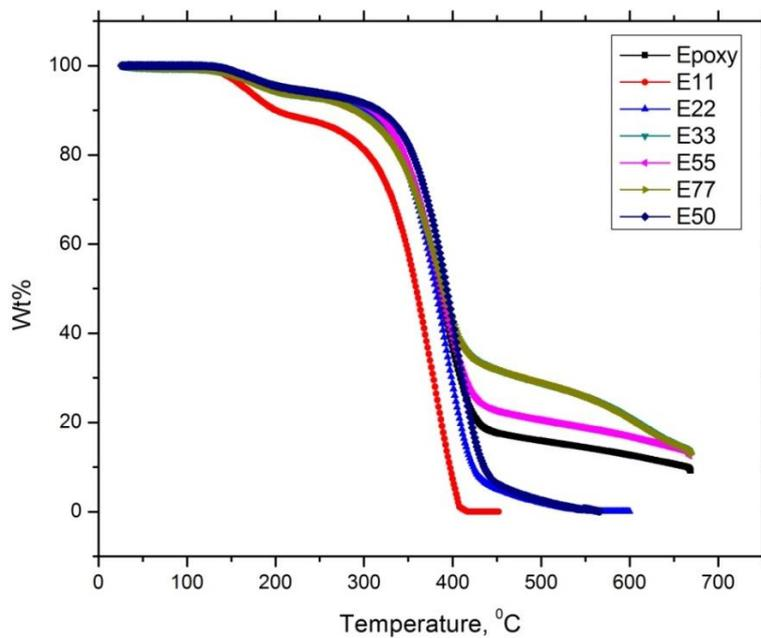
Fig. 6 Thermograms of epoxy-PP short fibers-clay composites
