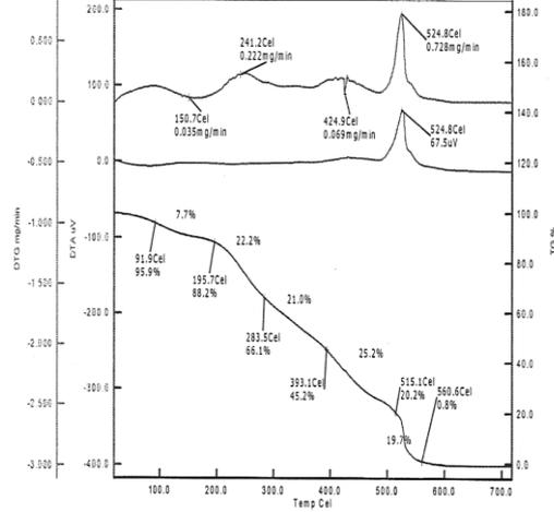
Fig. 3(b) Thermogram of (gelatin-co-PVA)-g-poly (AAc) copolymer
