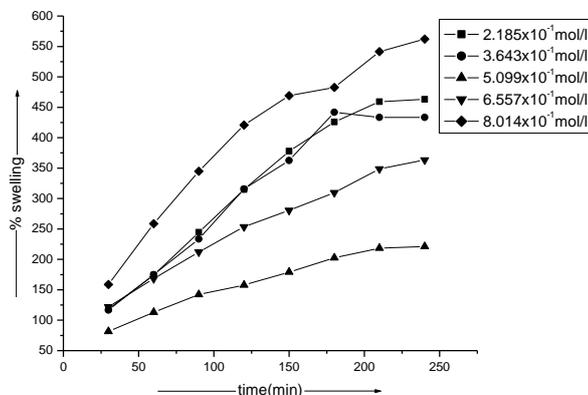
Fig. 1 Percentage of swelling of (gelatin-co-PVA)-g-poly(AAc) as a function of time: Effect of [AAc]
