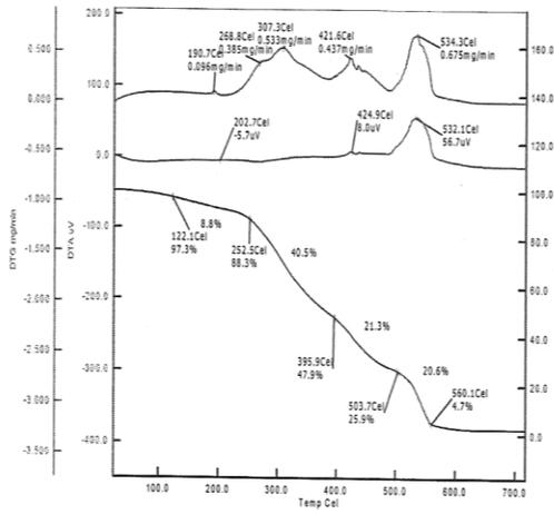
Fig. 3(a) Thermogram of gelatin-co-PVA copolymer
