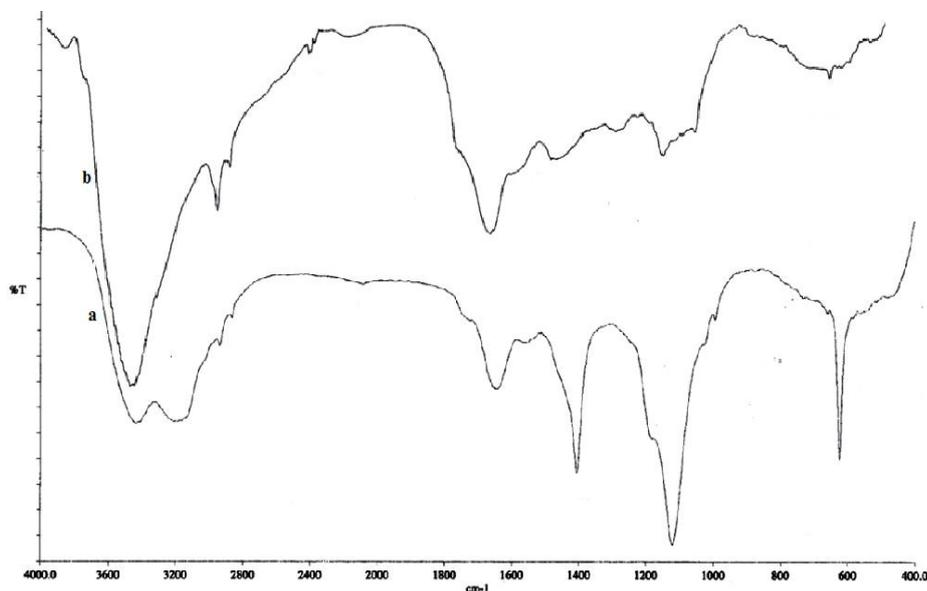
Fig. 2 FTIR of (a) gelatin-co-PVA and (b) (gelatin-co-PVA)-g-poly(AAc)
