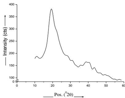
Fig.5(a) XRD pattern of the gelatin-co-PVA copolymer
