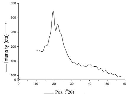
Fig.5(b) XRD pattern of the (gelatin-co-PVA)-g-poly (AAc) copolymer
