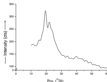
Fig.5(b) XRD pattern of the (gelatin-co-PVA)-g-poly (AAc) copolymer
