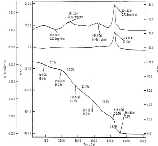
Fig. 3(b) Thermogram of (gelatin-co-PVA)-g-poly (AAc) copolymer
