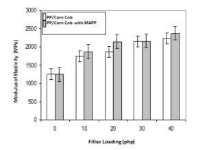
Fig. 5 The effect of filler loading on modulus of elasticity of uncompatibilized and compatibilized PP/CC biocomposites
