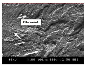
Fig. 9 The SEM micrograph of tensile fracture surface of compatibilized bicomposite (40 php corn cob)
