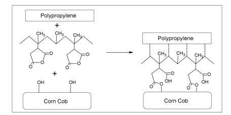
Fig. 3 Proposed schematic reaction between PP/corn cob biocomposite and MAPP
