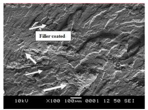
Fig. 8 The SEM micrograph of tensile fracture surface of compatibilized biocomposite (20 php corn cob)
