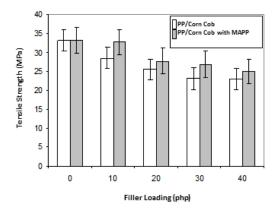
Fig. 2 The effect of filler loading on the tensile strength of uncompatibilized and compatibilized PP/CC biocomposites
