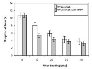
Fig. 4 The effect of filler loading on elongation at break of uncompatibilized and compatibilized PP/CC biocomposites
