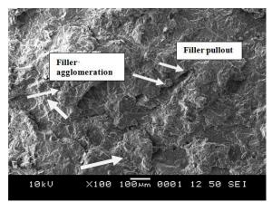
Fig. 7 The SEM micrograph of tensile fracture surface of uncompatibilized biocomposite (40 php corn cob)
