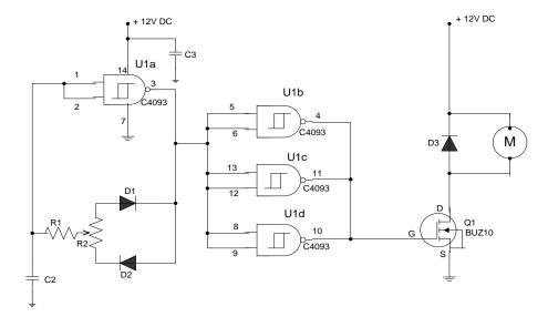
Fig. 2 Pulse width modulation (PWM) motor speed controller
