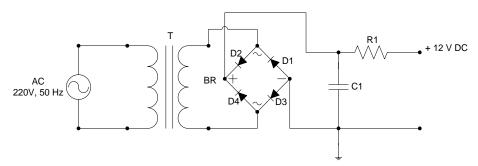
Fig. 1 Realization circuit of a DC Power Supply Circuit
