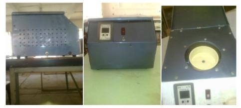
Fig. 4 Structure of the spin coater casing, (a) Side view and (b) front view
