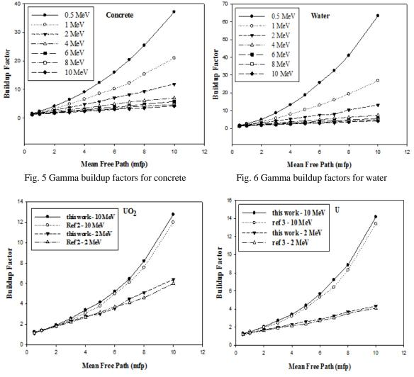
Fig. 7 Comparison of buildup factors obtained in this work with those of Ref. (Bozkurt and Tsoulfanidis 1996) for uranium dioxide (UO2) at 10 MeV
