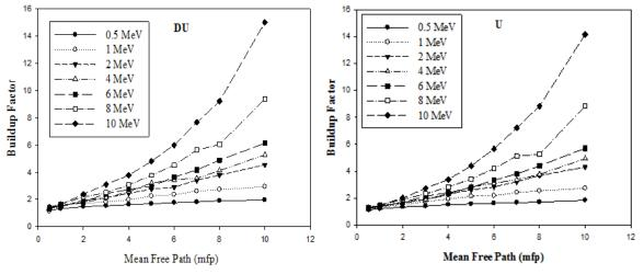
Fig. 1 Gamma buildup factors for depleted uranium (DU)
