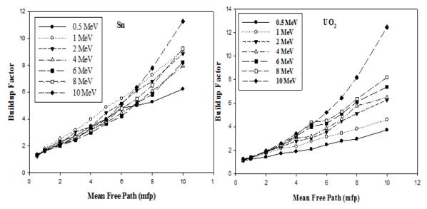
Fig. 3 Gamma buildup factors for tin
