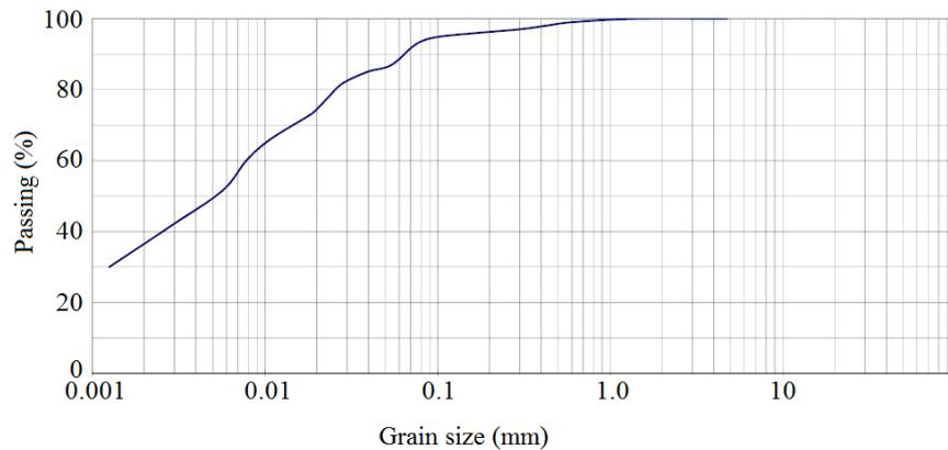
Fig. 2 The grain size analysis results for Tabriz landfill soil
