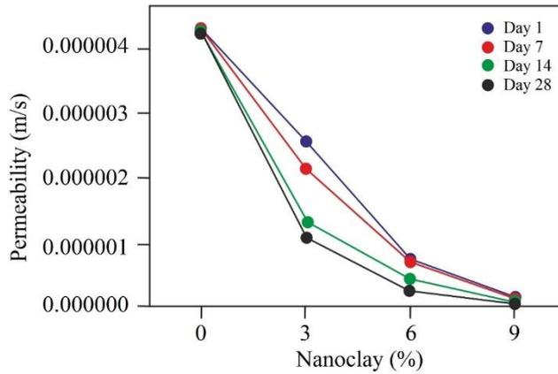
Fig. 4 Permeability variation in soil based on nanoclay content
