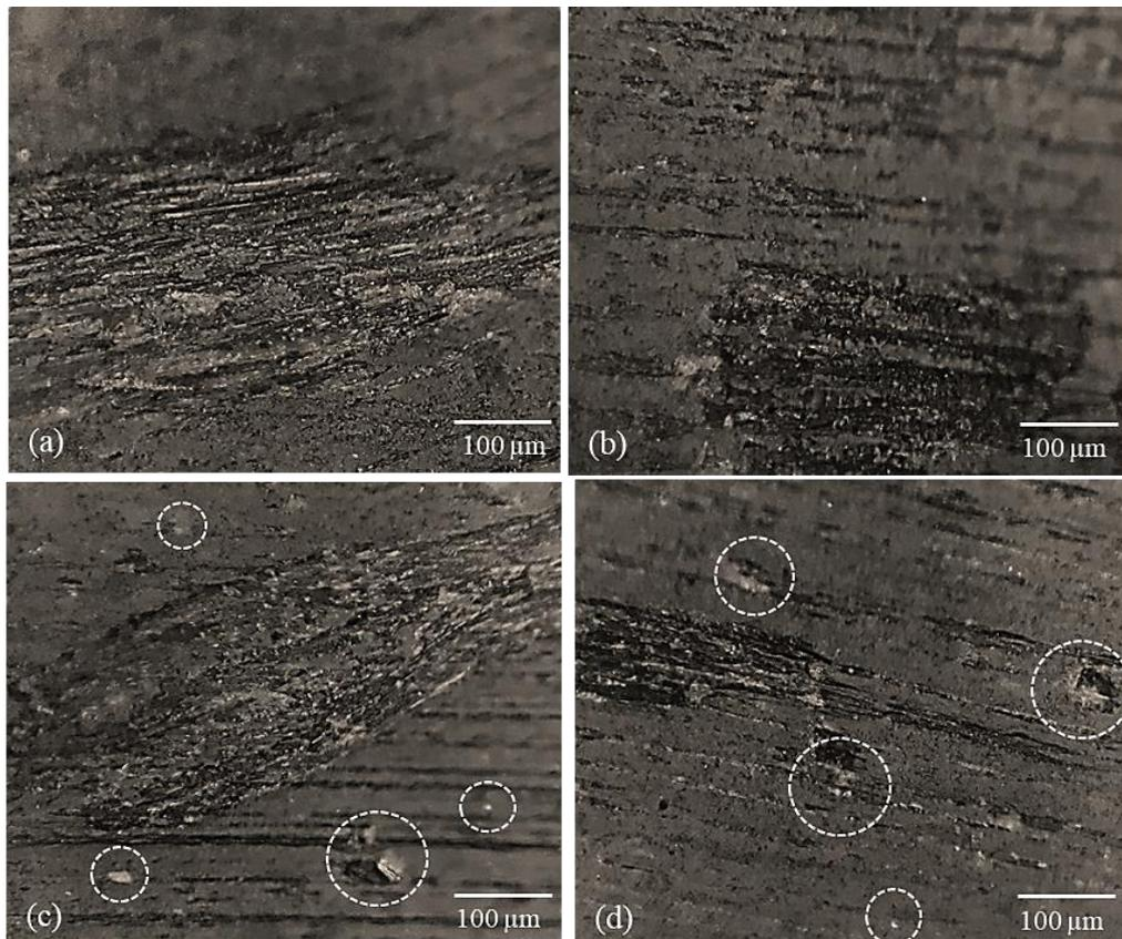
Fig. 8 Dispersion of fibres and particles in the matrix at 40x magnification: (a) rPP-10F, (b) rPP-20F, (c) rPP-10F-10G, and (d) rPP-20F-20G
