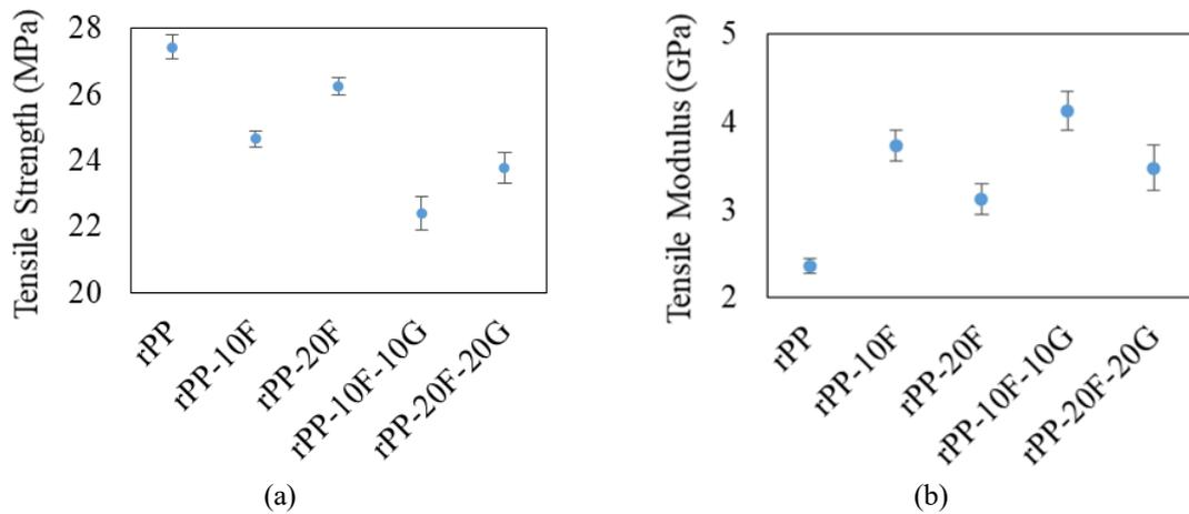
Fig. 3 Tensile properties of the experimental conditions: (a) tensile strength and (b) tensile modulus
