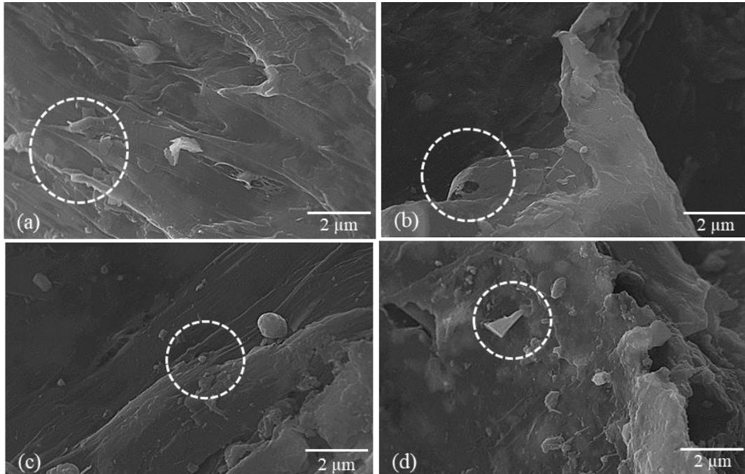
Fig. 9 Matrix-fibre-particle interface of the different composites tested (a) rPP-10F, (b) rPP-20F, (c) rPP-10F-10G, and (d) rPP-20F-20G. Magnification 2000x (30 kV)
