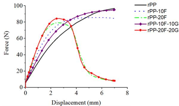
Fig. 6 Flexural tests: typical force-displacement curves
