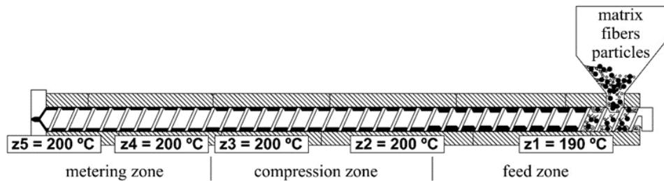
Fig. 2 Schematic diagram of the extruder, thread profile, and extrusion temperatures used
