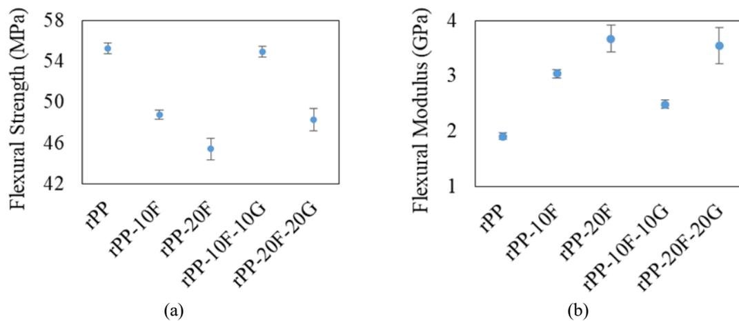
Fig. 5 Flexural properties of the experimental conditions: (a) tensile modulus and (b) flexural modulus
