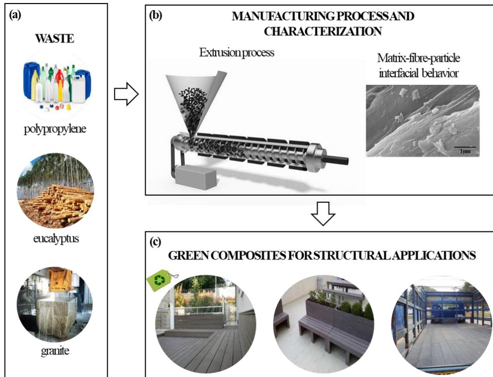
Fig. 1 Hybrid green composites with eucalyptus fibres and granite powder: (a) use of waste to produce composite materials, (b) manufacturing process by extrusion and interfacial adhesion analysis, and (c) structural applications of the new green composite
