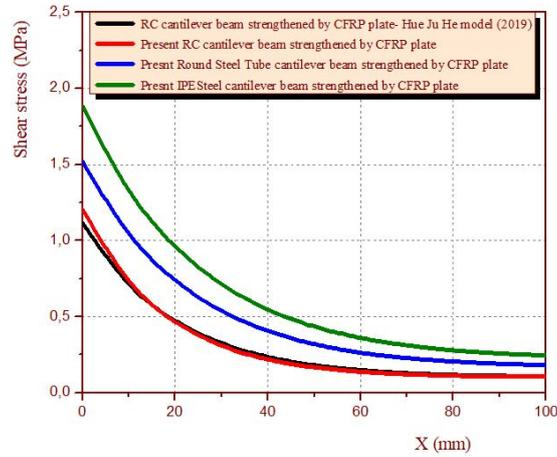
Fig. 5 Comparison of interfacial shear stress for CFRP-plated Steel cantilever beam with the analytical results
