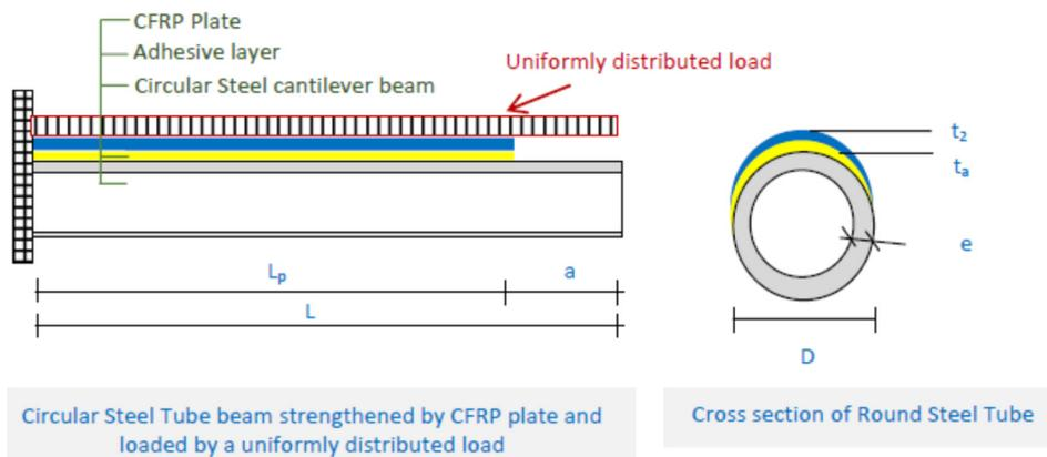
Fig. 1 Structure configuration of a circular steel beam strengthened by CFRP plate and loaded by a uniformly distributed load
