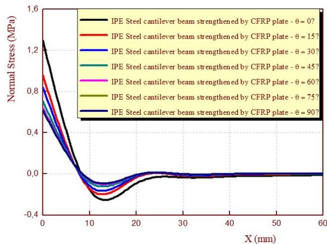
Fig. 10 Effect of the fiber orientation on the interfacial normal stresses for steel cantilever beam with a bonded CFRP soffit plate
