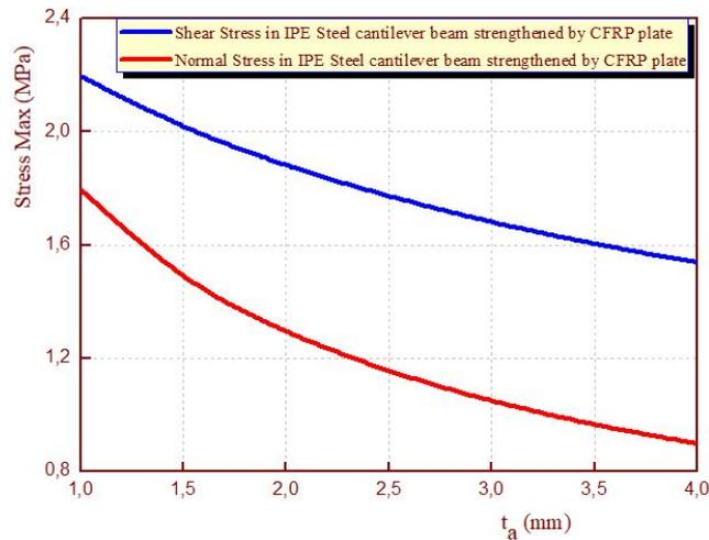
Fig. 13 Effect of Thickness of the adhesive layer on interfacial stresses
