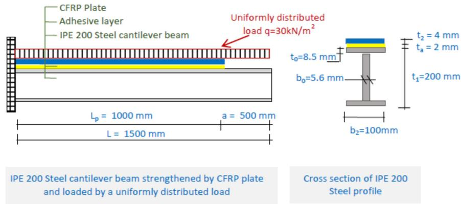
Fig. 3 IPE 200 Steel cantilever beam strengthened by CFRP plate and loaded by a uniformly distributed load
