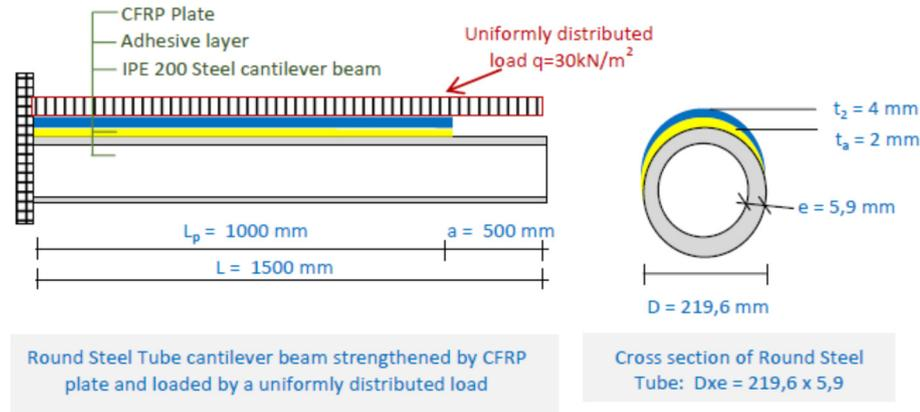
Fig. 4 Round Steel tube cantilever beam strengthened by CFRP plate and loaded by a uniformly distributed load
