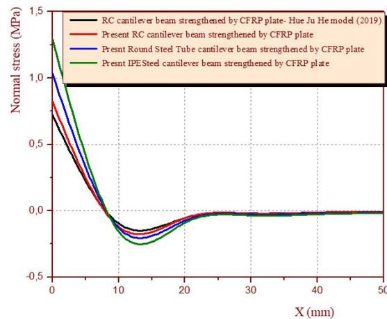
Fig. 6 Comparison of interfacial normal stress for CFRP-plated Steel cantilever beam with the analytical results
