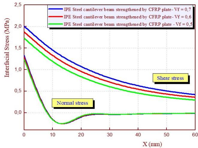
Fig. 11 Effect of fiber volume fraction on interfacial stresses
