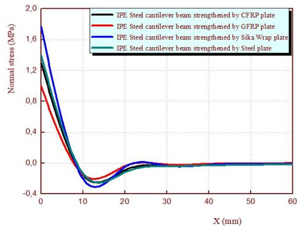
Fig. 8 Effect of plate stiffness on interfacial normal stresses
