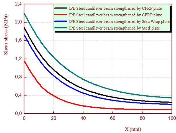
Fig. 7 Effect of plate stiffness on interfacial shear stresses
