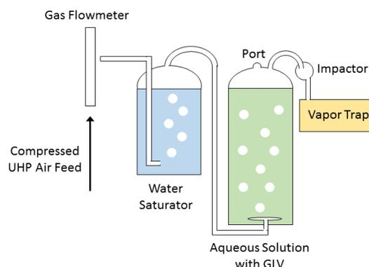
Fig. 2 Gas stripping apparatus for measurement of Henry's constant for GLVs
