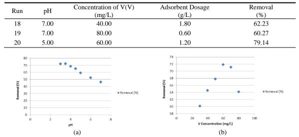
Fig. 4 (a) Effects of pH on removal efficiency and (b) Effects of initial concentration of vanadium(V) on removal efficiency
