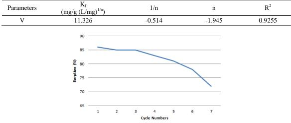
Fig. 7 Elution operation with 0.01 M HCl after V adsorbed onto the composite adsorbent
