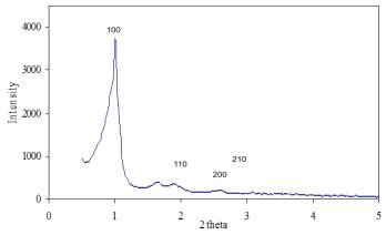
Fig. 4 X-ray diffraction pattern of SBA-15
