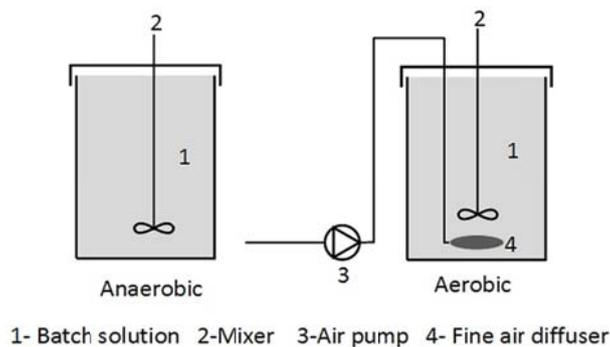
Fig. 1 Schematic diagram of the anaerobic and the aerobic jars
