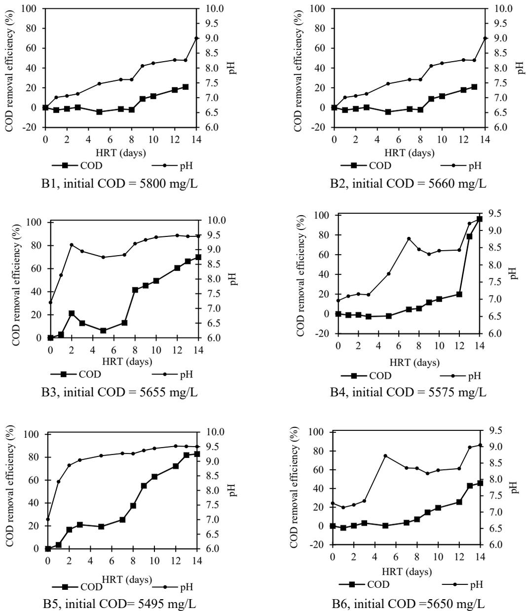
Fig. 3 COD removal efficiency vs. time at granule dose of 0.4 g/L
