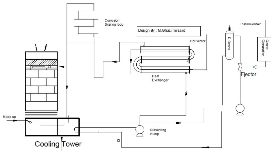
Fig. 1 Block diagram for the ozone treatment pilot plant
