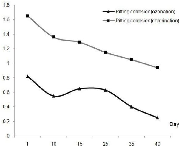
Fig. 4 Pitting corrosion plot in the two treatment methods
