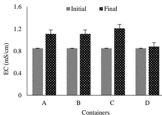
Fig. 6 Comparison of electrical conductivity variation in different containers
