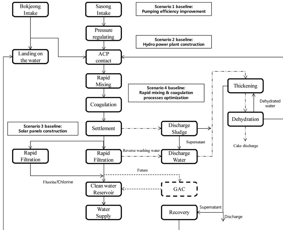
Fig. 1 Scheme of project baseline on S-WTS
