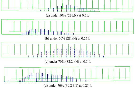
Fig. 3 Crack pattern of RC beam under different damage load located at different distance from left support (Cracks are shown in blue and red)
