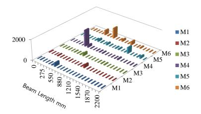
Fig. 16 MCDF for beam under 70% UL (39.2 8kN) located at 550 mm from left support, for mode shapes M1 to M6  $\,$
