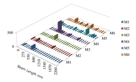
Fig. 14 MCDF for beam under 50% UL (238kN) located at 550 mm from left support, for mode shapes M1 to M6
