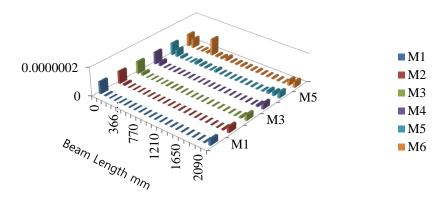
Fig. 12 LSI for beam under 70% UL (39.2 kN) located at 550 mm from left support, for mode shapes M1 to M6  $\,$
