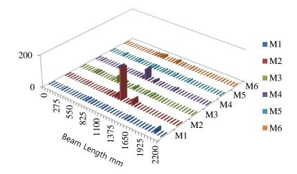
Fig. 21 MLSI for beam under 70% UL (32.2 KN) located at 1100 mm from left support, for mode shapes M1 to M6  $\,$
