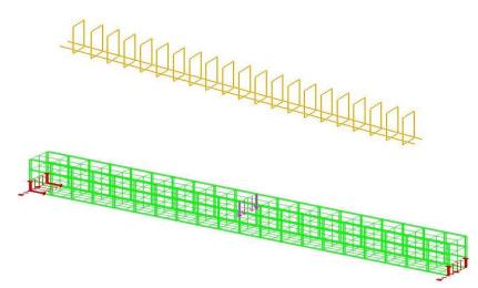
Fig. 2 Finite element model of reinforced concrete beam (top: reinforced bars modelling; bottom: concrete beam modelling) – Orange colour is reinforcement elements, green colour is concrete brick elements, red colour is support restrains, and burble colour is applied load
