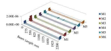
Fig. 9 LSI for beam under 50% UL (23kN) located at 1100 mm from left support, for mode shapes M1 to M6
