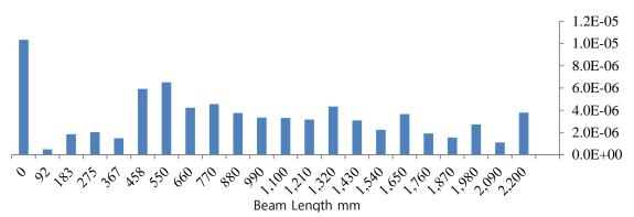
Fig. 7 CDF for beam under 70% UL (39.2 kN) located 550 mm from left support
