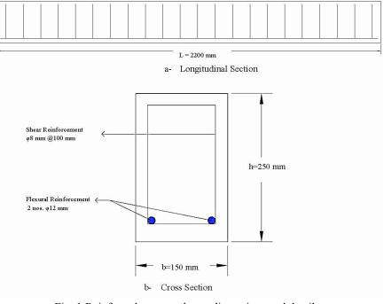
Fig. 1 Reinforced concrete beam dimensions and details
