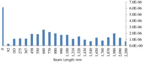
Fig. 5 CDF for beam under 50% UL (28 kN) located 550 mm from left support
