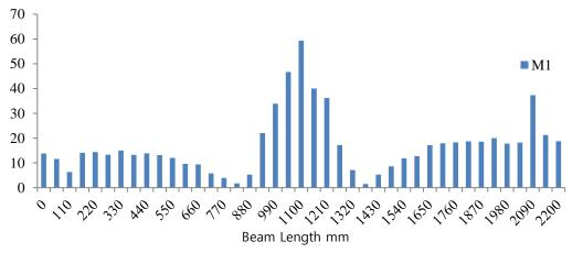
Fig. 18 MCDF for Mode 1 of beam under 70%UL (32.2 kN) located at 1100 mm from left support
