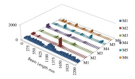
Fig. 23 MCDF for beam under 50% UL (23 KN) located at 1100 mm by using Fourier Estimation, for mode shapes M1 to M6
