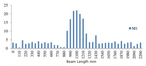
Fig. 17 MCDF for Mode 1 of beam under 50% UL (23 8kN) located at 1100 mm from left support
