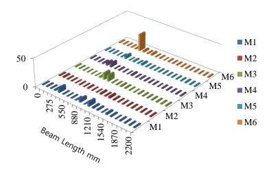
Fig. 22 MLSI for beam under 70% UL (39.2 KN) located at 550 mm from left support, for mode shapes M1 to M6
