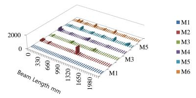
Fig. 13 MCDF for beam under 50% UL (23kN) located at 1100 mm from left support, for mode shapes M1 to M6
