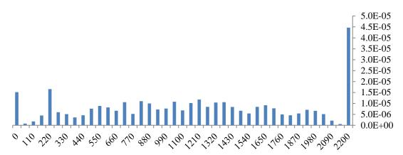
Beam Length mm Fig. 6 CDF for beam under 70% UL (32.2 kN) located 1100 mm from left support
