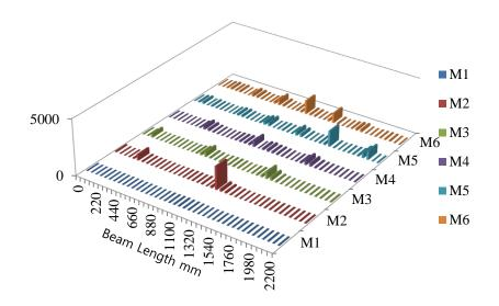
Fig. 15 MCDF for beam under 70% UL (32.2 8kN) located at 1100 mm from left support, for mode shapes M1 to M6
