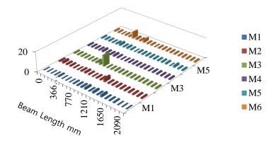
Fig. 20 MLSI for beam under 50% UL (28 KN) located at 550 mm from left support, for mode shapes M1 to M6
