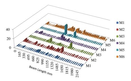
Fig. 24 MLSI for beam under 50% UL (23 KN) located at 1100 mm by using Fourier Estimation, for mode shapes M1 to M6
