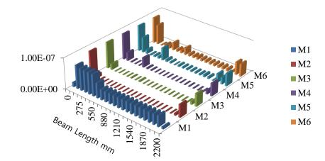
Fig. 10 LSI for beam under 50% UL (28 kN) located at 550 mm from left support, for mode shapes M1 to M6  $\,$
