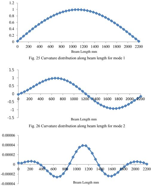
Fig. 27 Curvature distribution along beam length for modes 3
